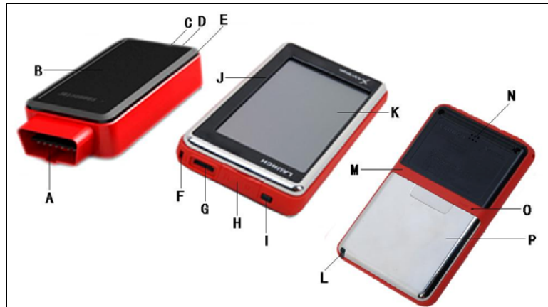
Figure 2-2 X-431Diagun main unit ports and indicators
