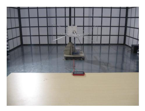
Radiation Emission Test Setup (Above 1GHz)
