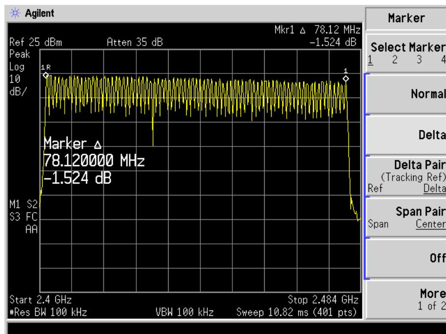
Channel Spacing (Low CH=1MHz)
