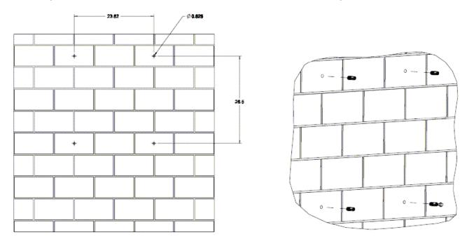
DRILL 4 Ø 5/8" HOLES INTO WALL TO A DEPTH OF 1.75", AS DETAILED ABOVE
