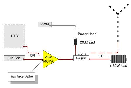
Figure 5 – Recommended Test Setup
