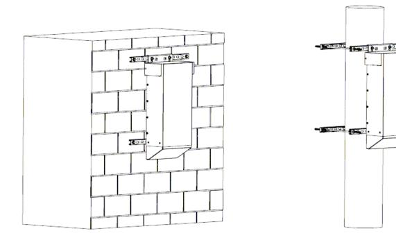
Figure 3 – Wall mount or pole mount installation
