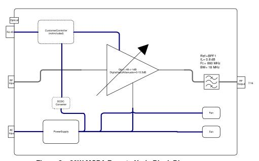
Figure 2 – 20W MCPA Remote Node Block Diagram
