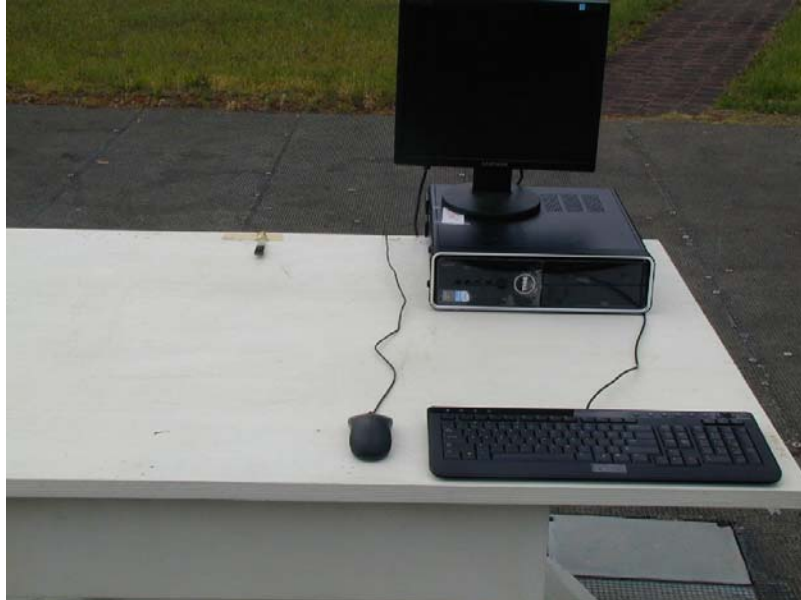
FCC Part 15C Radiated Disturbance Test Setup (Front View – EUT Transmit Mode)
