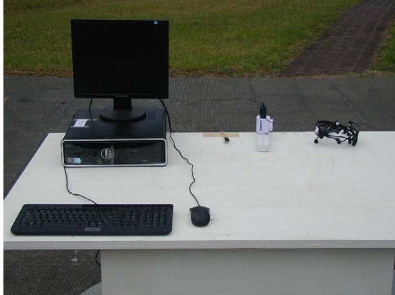
FCC Part 15B Radiated Disturbance Test Setup (Front View – EUT Charging Mode)
