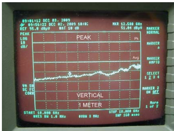
Radiated Emissions Plot (V-Pol, 10GHz-18GHz)
