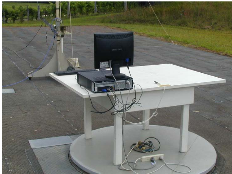
FCC Part 15C Radiated Disturbance Test Setup (Rear View – EUT Transmit Mode)
