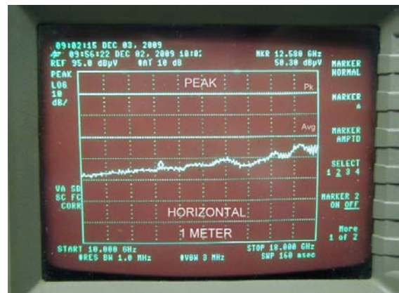
Radiated Emissions Plot (H-Pol, 10GHz-18GHz)
