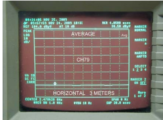
Field Strength Plot (CH79, H Pol, Average)
