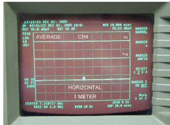
Radiated Emissions Plot (CH4 3 rd Har, H-Pol, Average)
