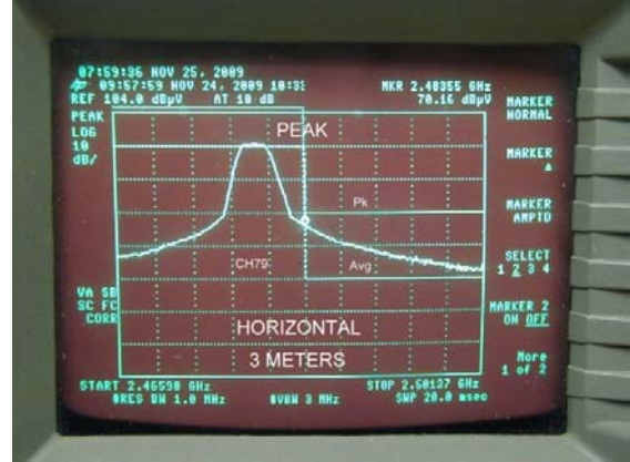
Radiated Emissions Plot (CH79, H-Pol, Peak)
