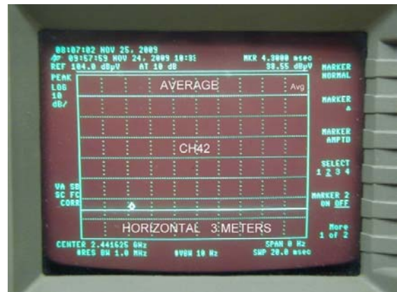
Field Strength Plot (CH42, H Pol, Average)
