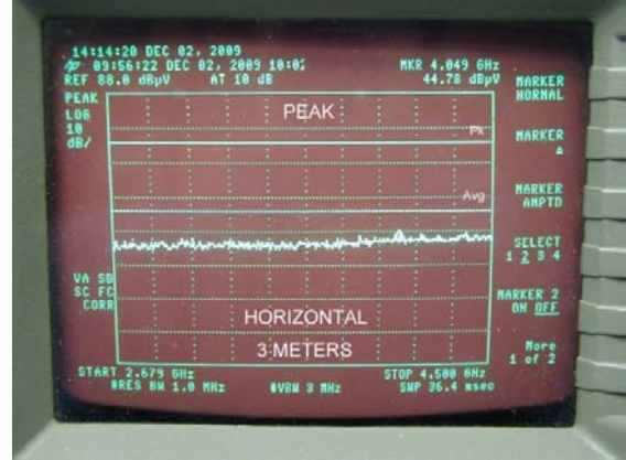
Radiated Emissions Plot (H-Pol, 2.68GHz-4.5GHz)
