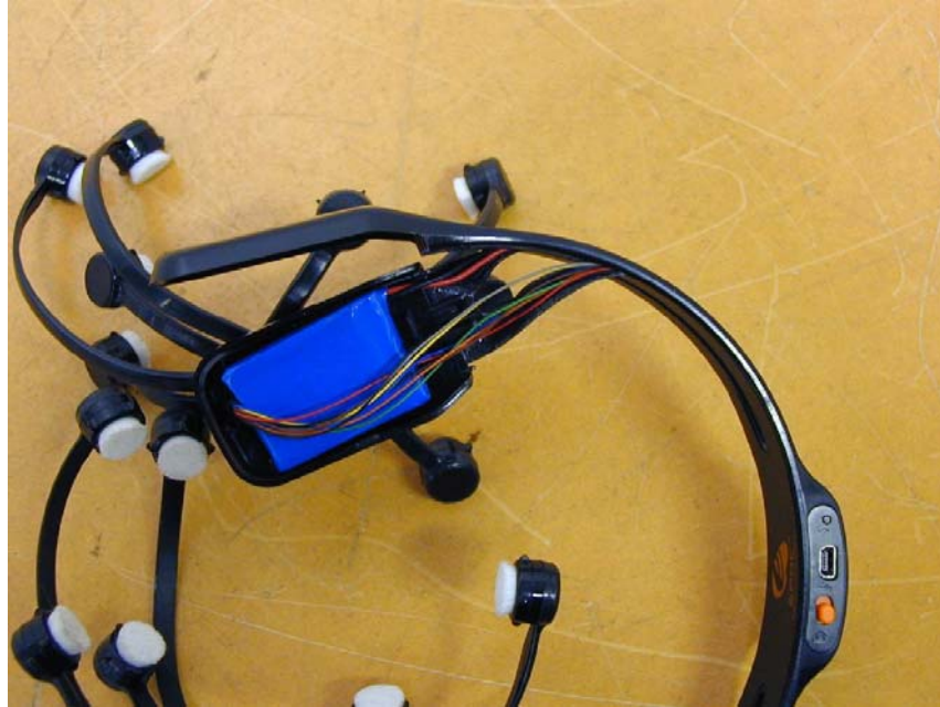
EUT Left Side (Internal Battery View)
