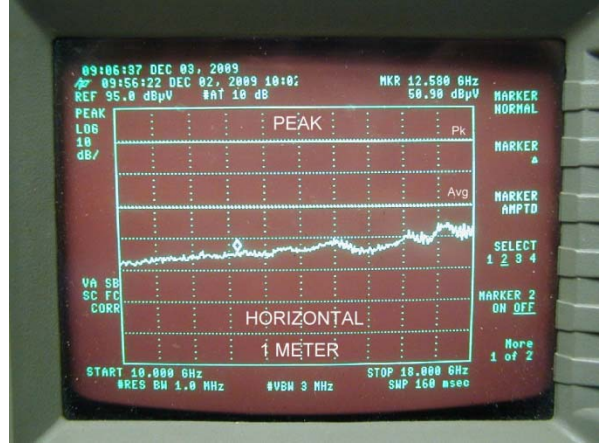
Radiated Emissions Plot (H-Pol, 10GHz-18GHz)
