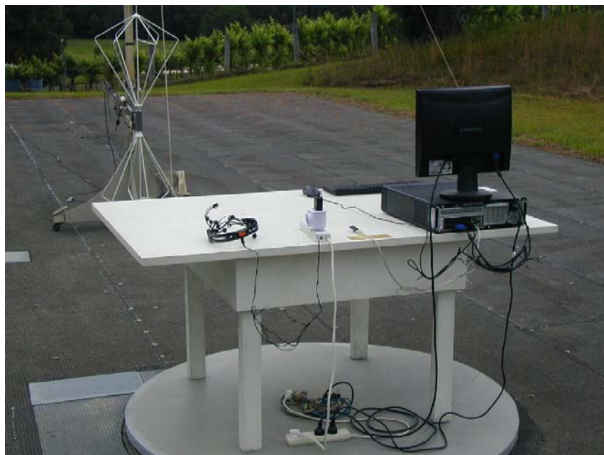
FCC Part 15B Radiated Disturbance Test Setup (Rear View – EUT Charging Mode)
