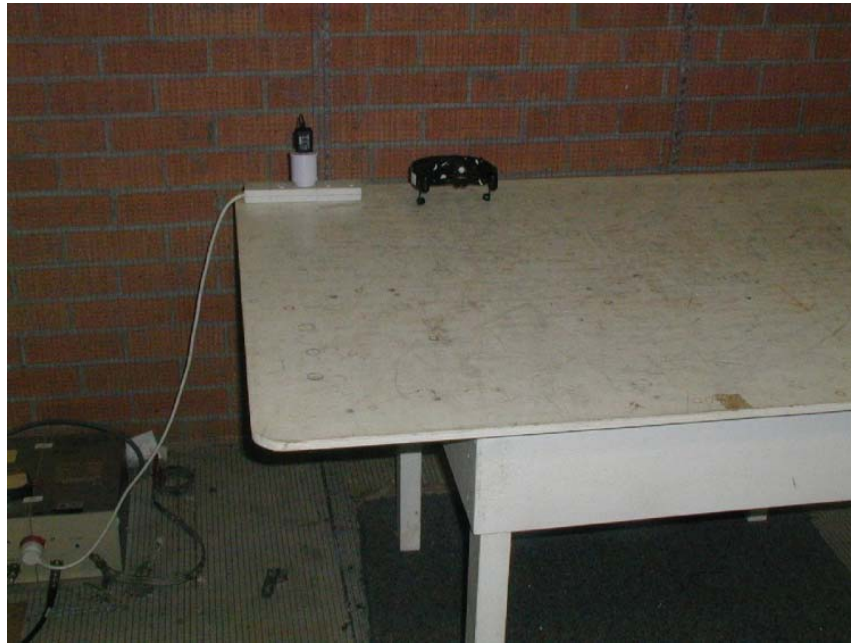
Conducted Disturbance Test Setup (Front View)
