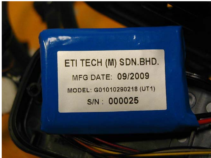
EUT Internal Battery
