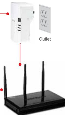
2. Connect a network cable from the powerline adapter to an available LAN network port on your router (e.g. TEW-691GR).
