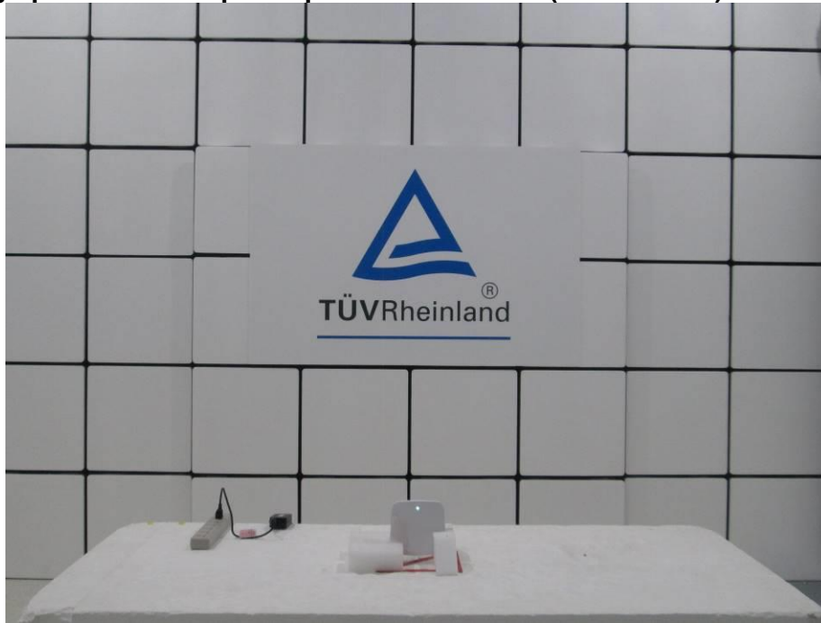
Photograph 10: Test Setup for Spurious Emissions (Front View 2)
