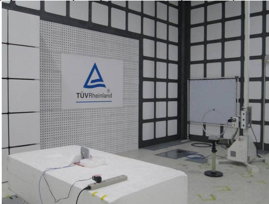
Photograph 4: Test Setup for Spurious Emissions (Back View 2)
