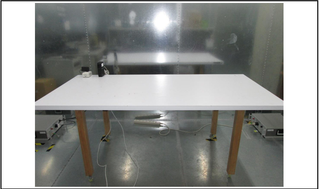
Conducted Emission Test _ Test Configuration 1
