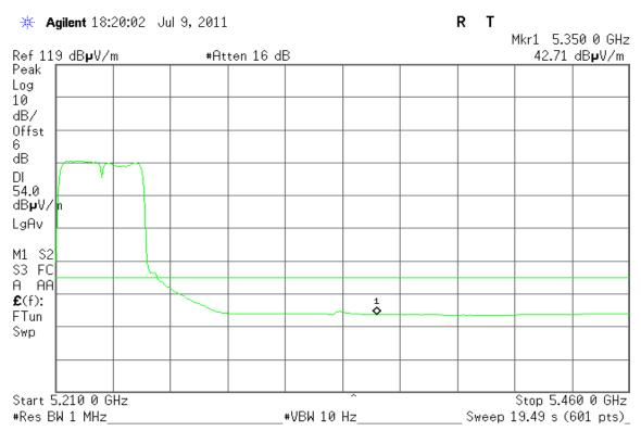
Detector mode: Peak Polarity: Horizontal
