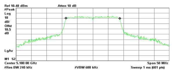
Occupied Bandwidth 17.4647 MHz Occ BW % Pwr 99.00 % x dB -26.00 dB
