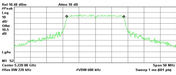
Occupied Bandwidth 17.5066 MHz Occ BW % Pwr 99.00 % x dB -26.00 dB
