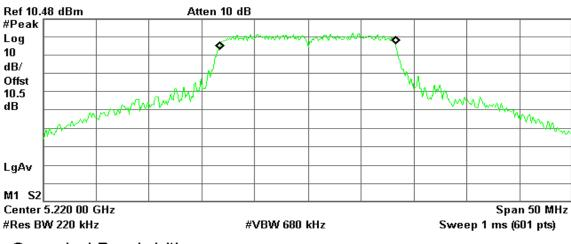
Occupied Bandwidth 16.5290 MHz Occ BW % Pwr 99.00 % x dB -26.00 dB
