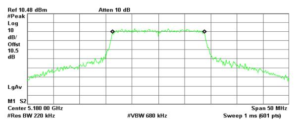
Occupied Bandwidth 17.4727 MHz Occ BW % Pwr 99.00 % x dB -26.00 dB
