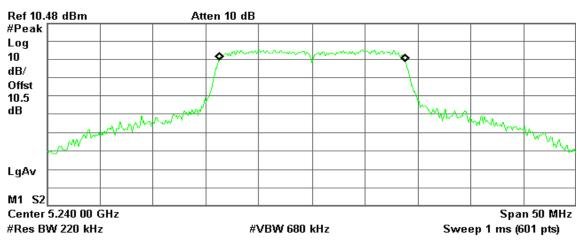
Occupied Bandwidth 17.4454 MHz Occ BW % Pwr 99.00 % x dB -26.00 dB
