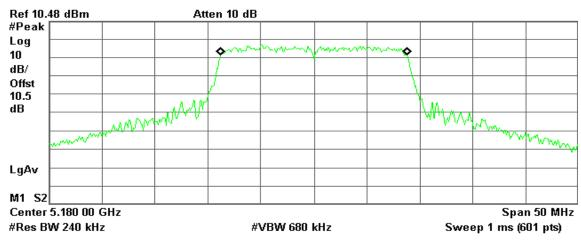
Occupied Bandwidth 17.4991 MHz Occ BW % Pwr 99.00 % x dB -26.00 dB
