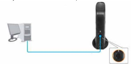
2. Plug in the power adapter and verify the Power & Ethernet LEDs are light.
