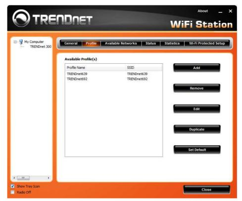
**Add:** Adds a profile. The following screen will appear. The user can enter the necessary information required for accessing the particular Access Point or Wireless Router. Or you can search the desire wireless router or AP under **Available Networks** section and click on **Add Profile** button to add the Profile.
