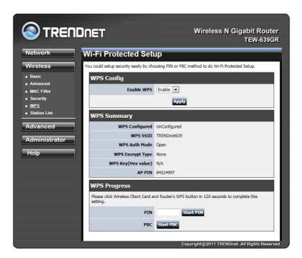
3) Choose to select the specific AP/Router or a WPS enabled device with client PIN entered.
