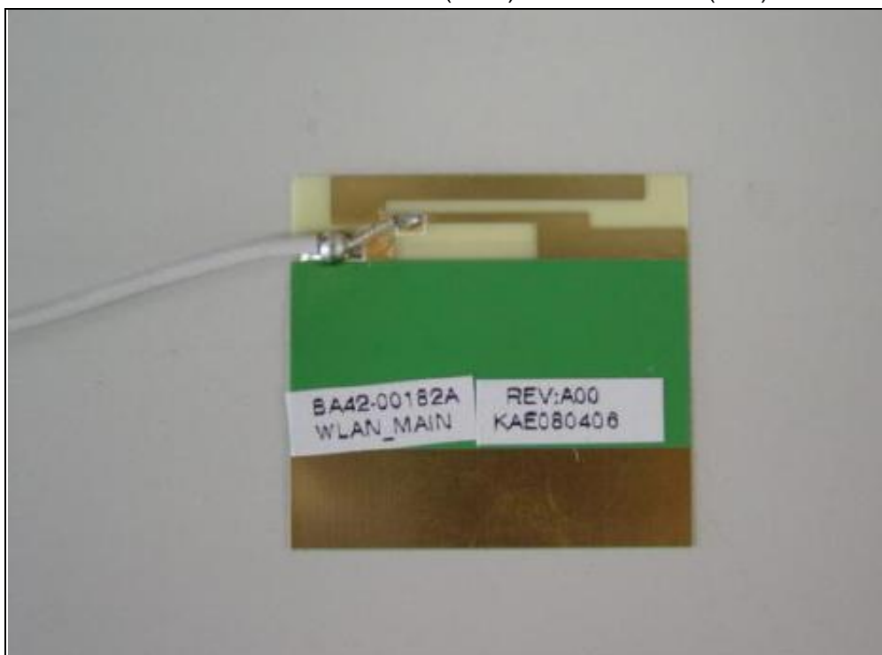
Antenna 45: SS-03-03-099 (Main) / SS-03-03-100 (Aux)
