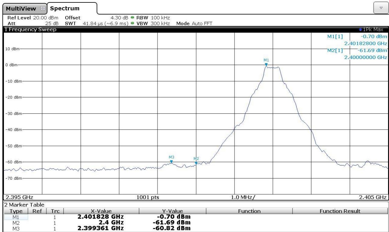
**Band-edge Compliance of RF Emissions, GFSK (Hopping On) – Lower Band Edge**
