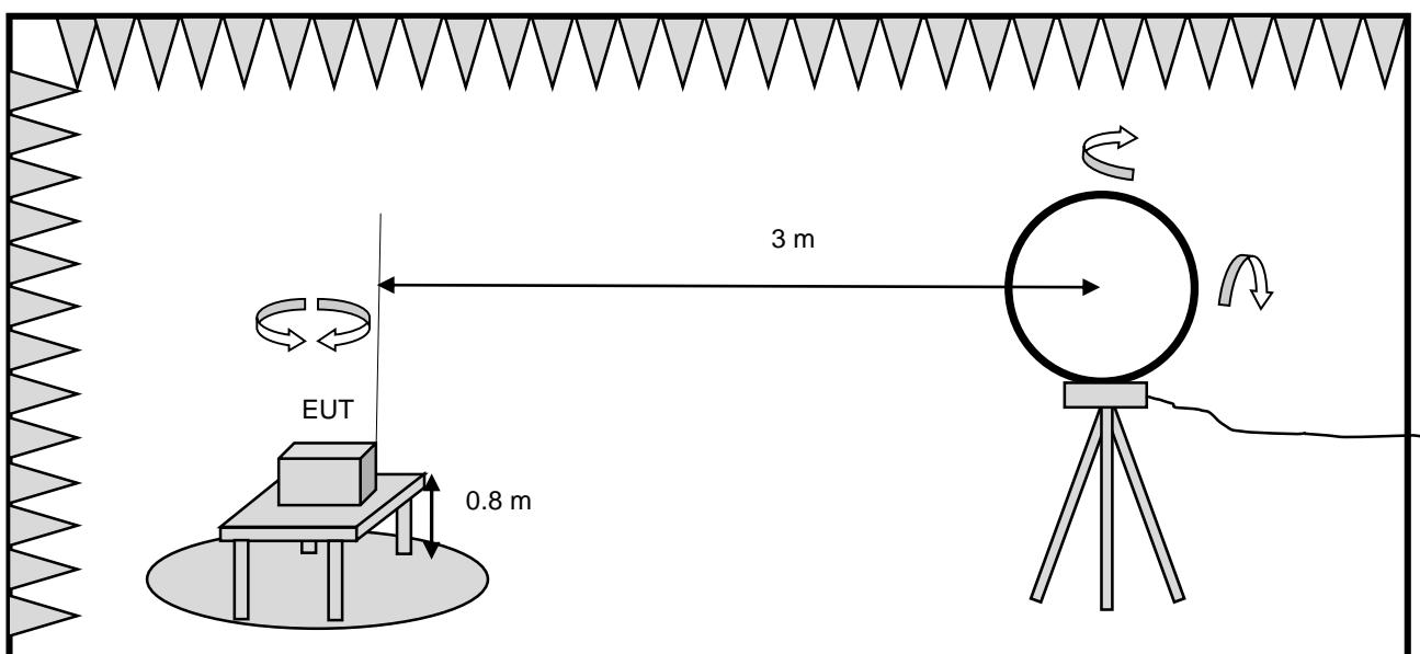
Semi anechoic chamber with absorber and ferrite tiles
