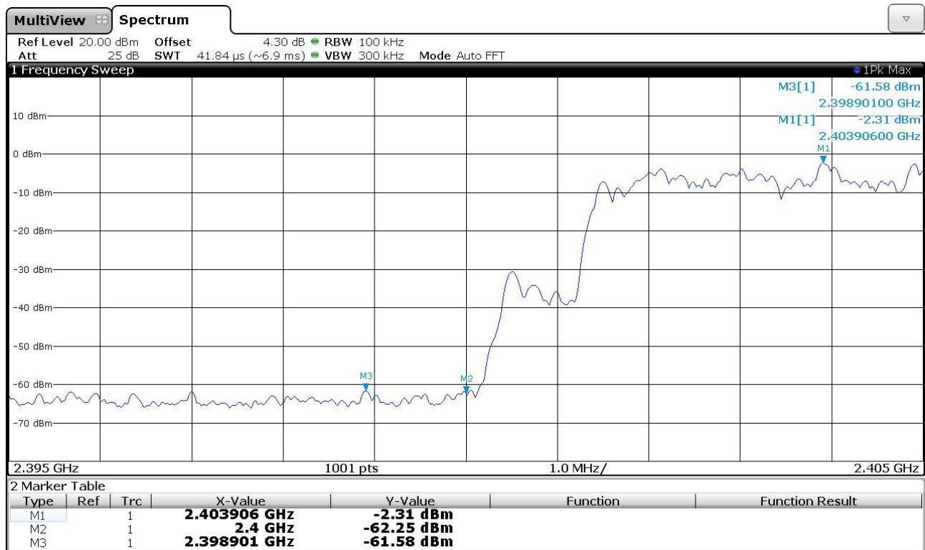
**Band-edge Compliance of RF Emissions,  $\pi/4$ -DQPSK (Hopping Off) – Upper Band Edge**
