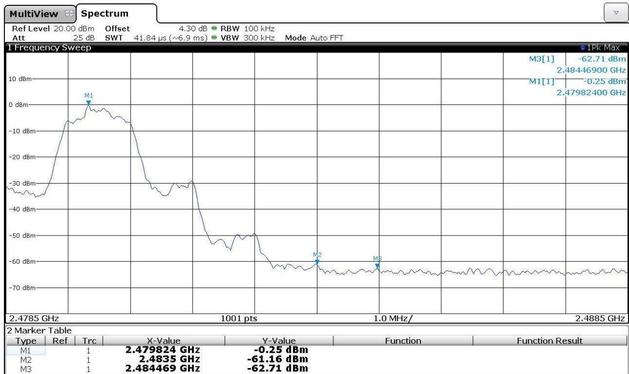
**Band-edge Compliance of RF Emissions,  $\pi/4$ -DQPSK (Hopping On) – Upper Band Edge**
