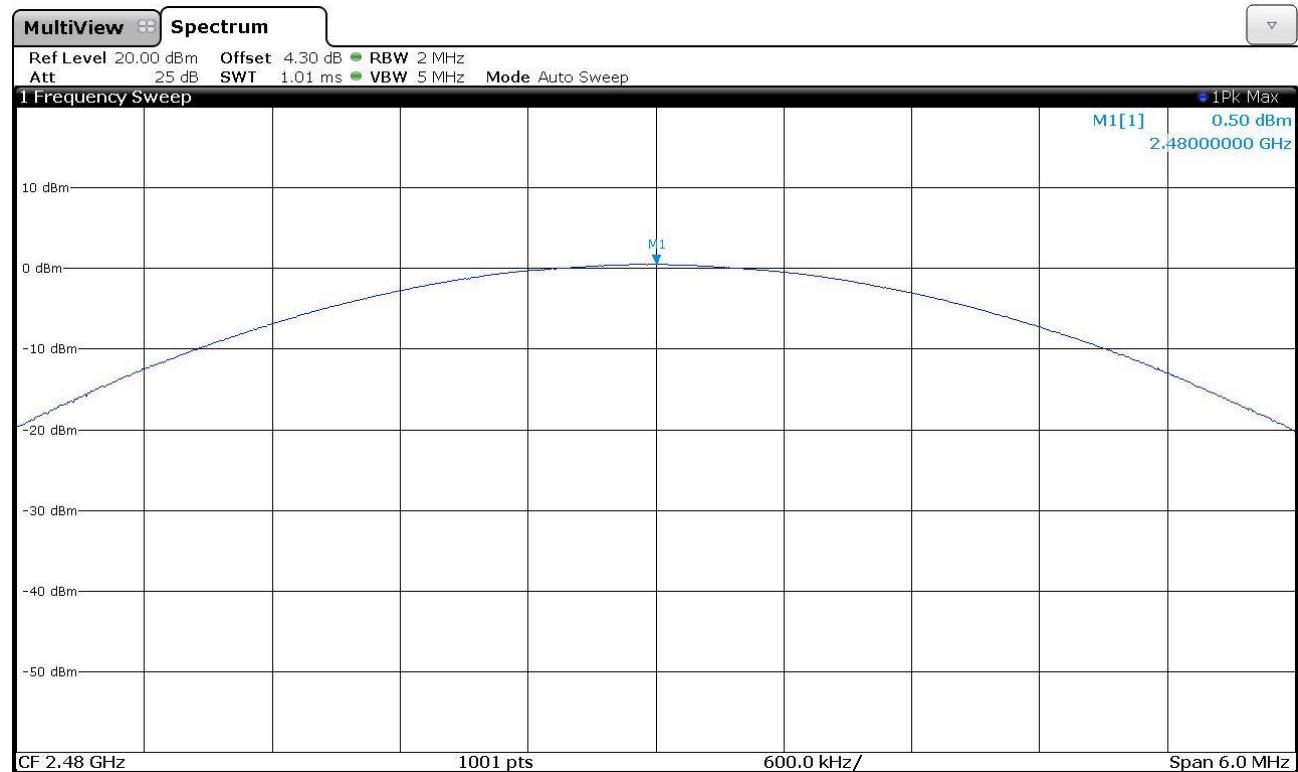
**Results of Bluetooth Communication mode (8DPSK) (Fundamental Power):
