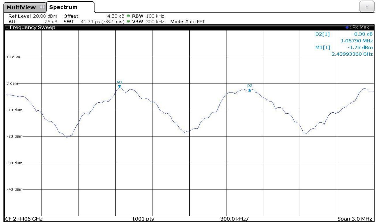
**Highest Operating Frequency - GFSK**
