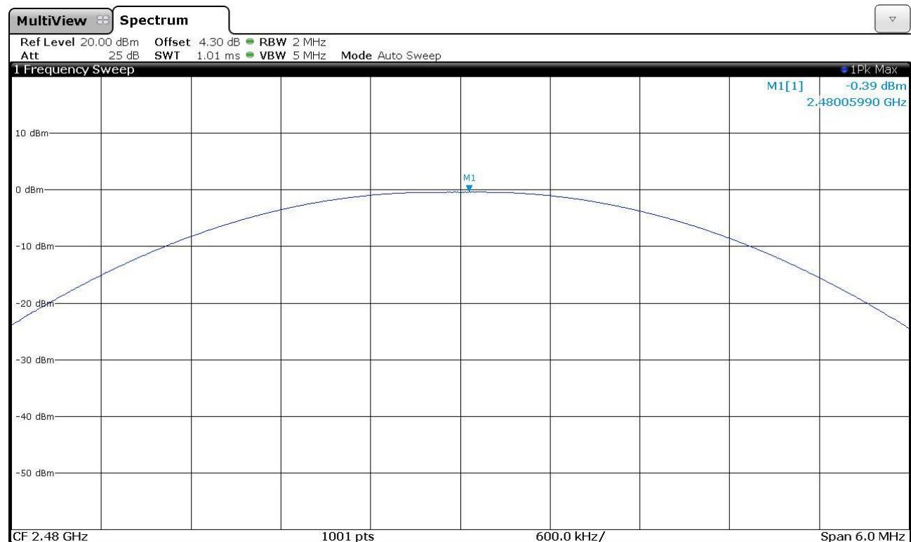
**Results of Bluetooth Communication mode (GFSK) (Fundamental Power):
