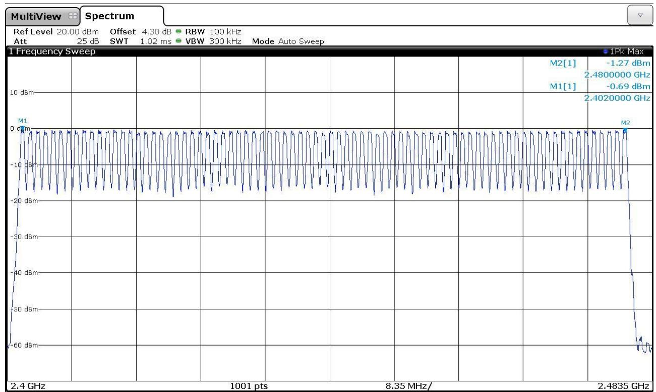
**$\pi/4$ -DQPSK: 79 of 79 Channel**
