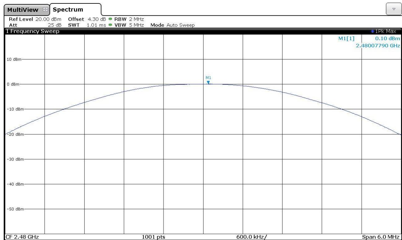
**Results of Bluetooth Communication mode ( $\pi/4$ -DQPSK) (Fundamental Power):
