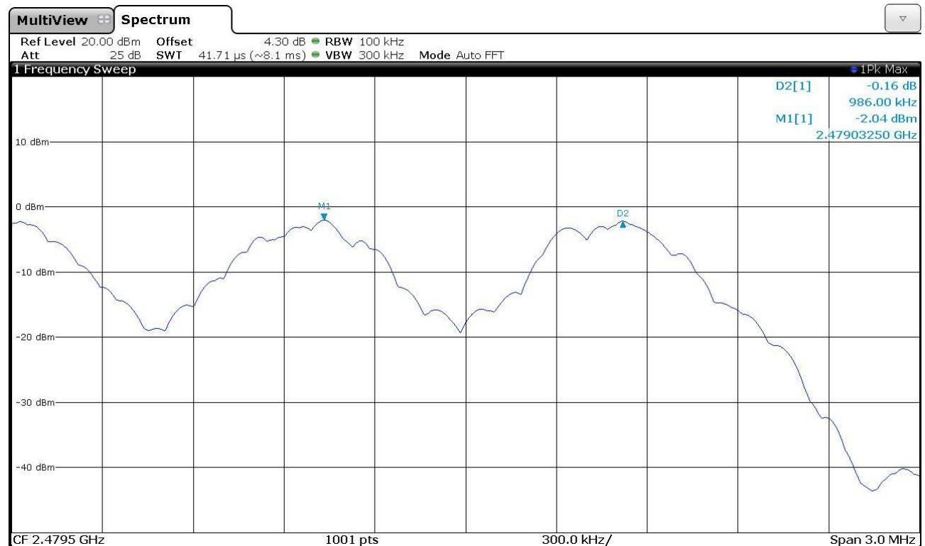
**Summary of Channel separation measurements - GFSK**
