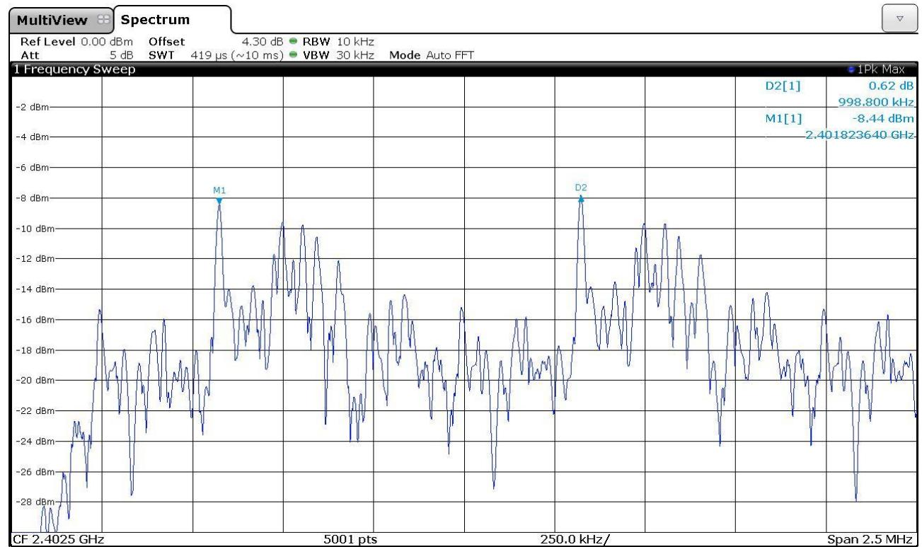
Middle Operating Frequency –  $\pi/4$  DQPSK
