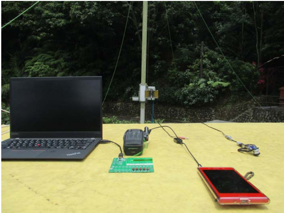
Above 1 GHz (EUT at 1.5m)
