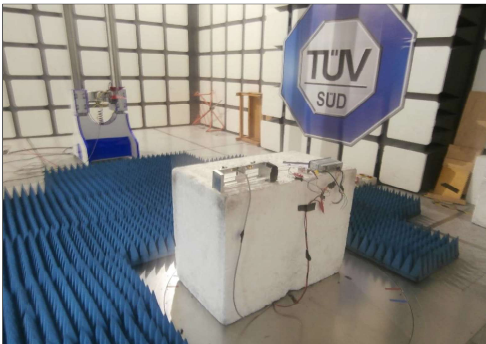
Figure 11 - Test Setup - Above 1 GHz
