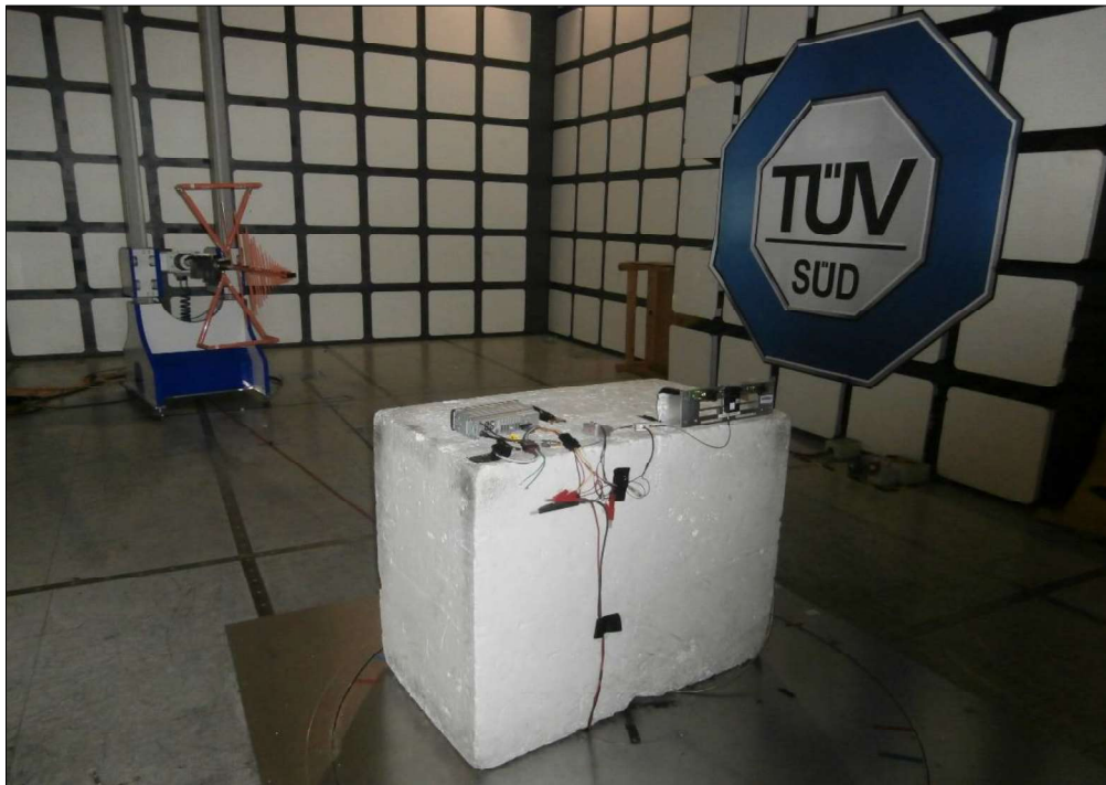
Figure 10 - Test Setup - Below 1 GHz
