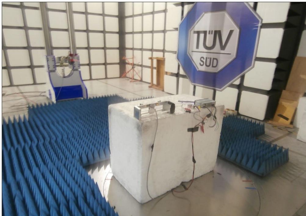
Figure 11 - Test Setup - Above 1 GHz
