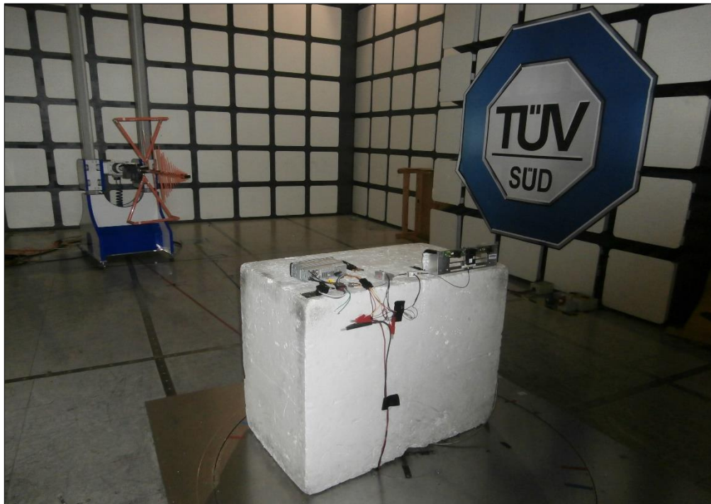
Figure 10 - Test Setup - Below 1 GHz
