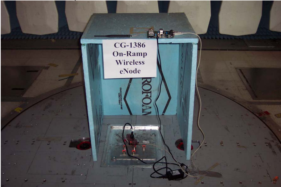
Radiated Emission setup with 5dBi Antenna Vertical
