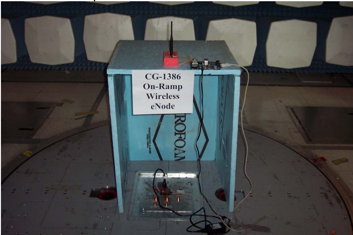
Radiated Emission setup with 5dBi Antenna Vertical
