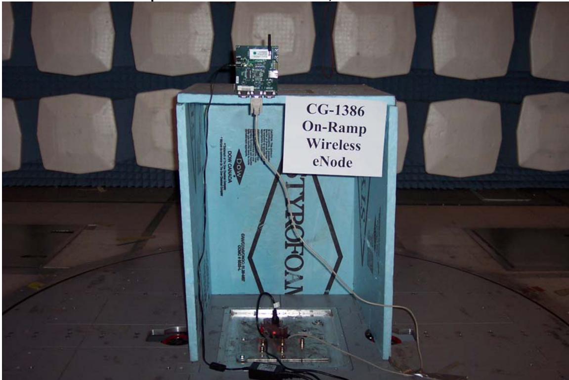
Radiated Emission setup with 1dBi Antenna Vertical, EUT Vertical
