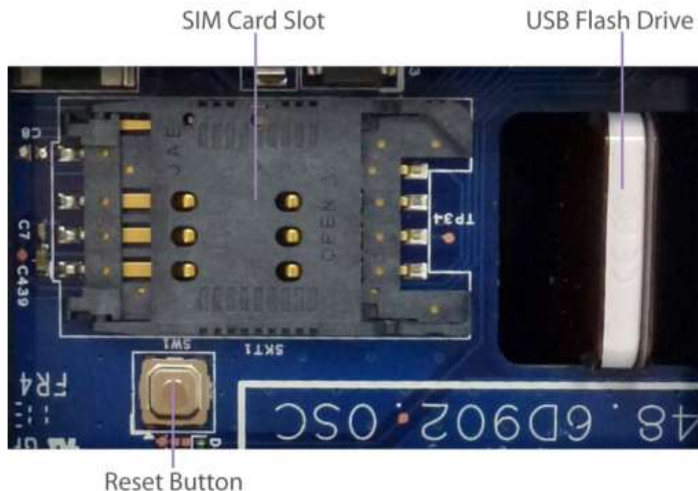
Figure 3-3 – SIM Card Slot, USB Flash Disk, and Reset Button Locations
