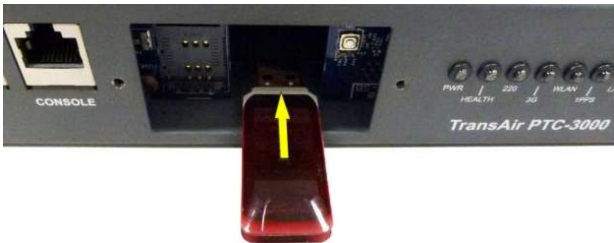
Figure 4-4 – USB Flash Drive Installation (1U unit shown)
