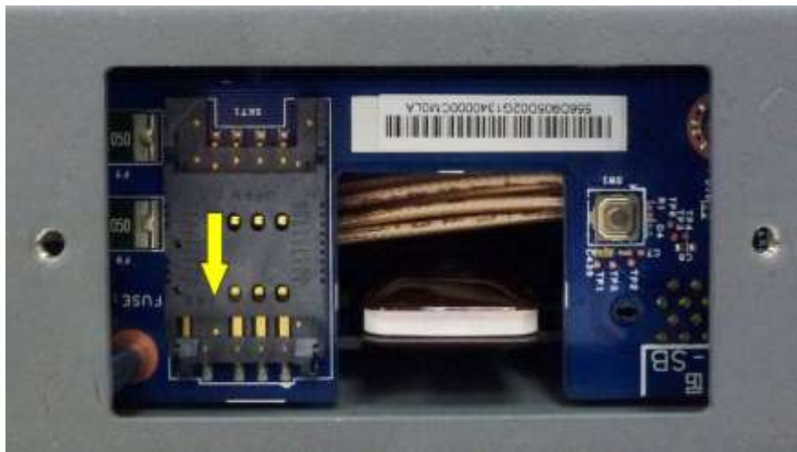
Figure 4-6 – Slide SIM Card Slot Protective Cover Down
