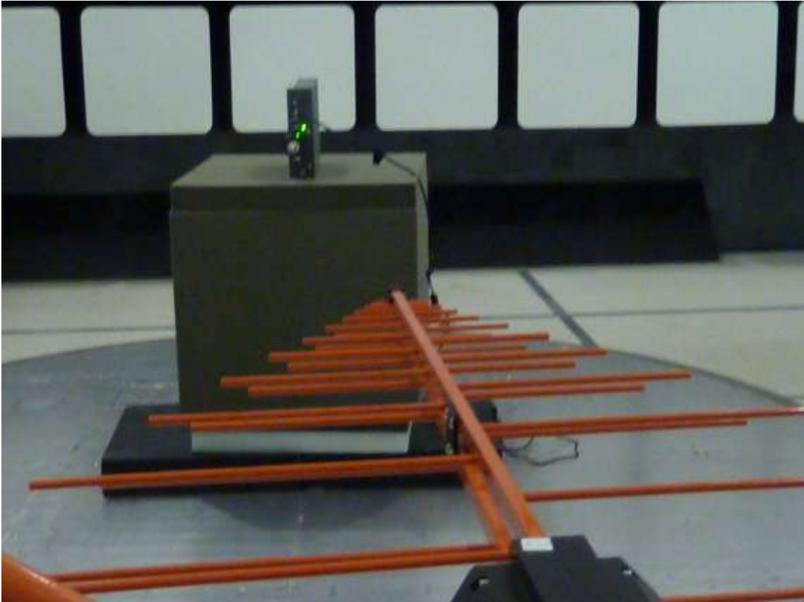
Radiated Emissions Front side
