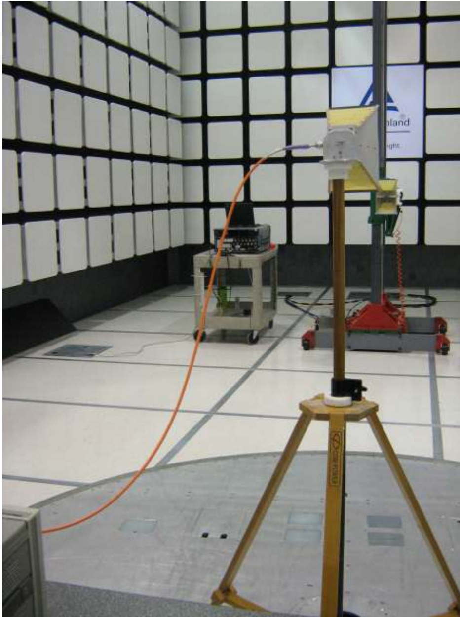
Photo of Test Setup for 1 GHz to 2.5 GHz Substitution
