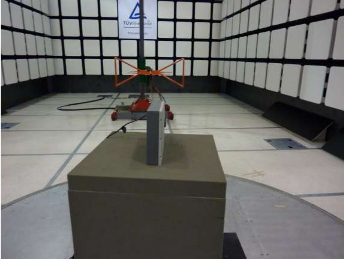
Test Setup – Radiated Emissions
