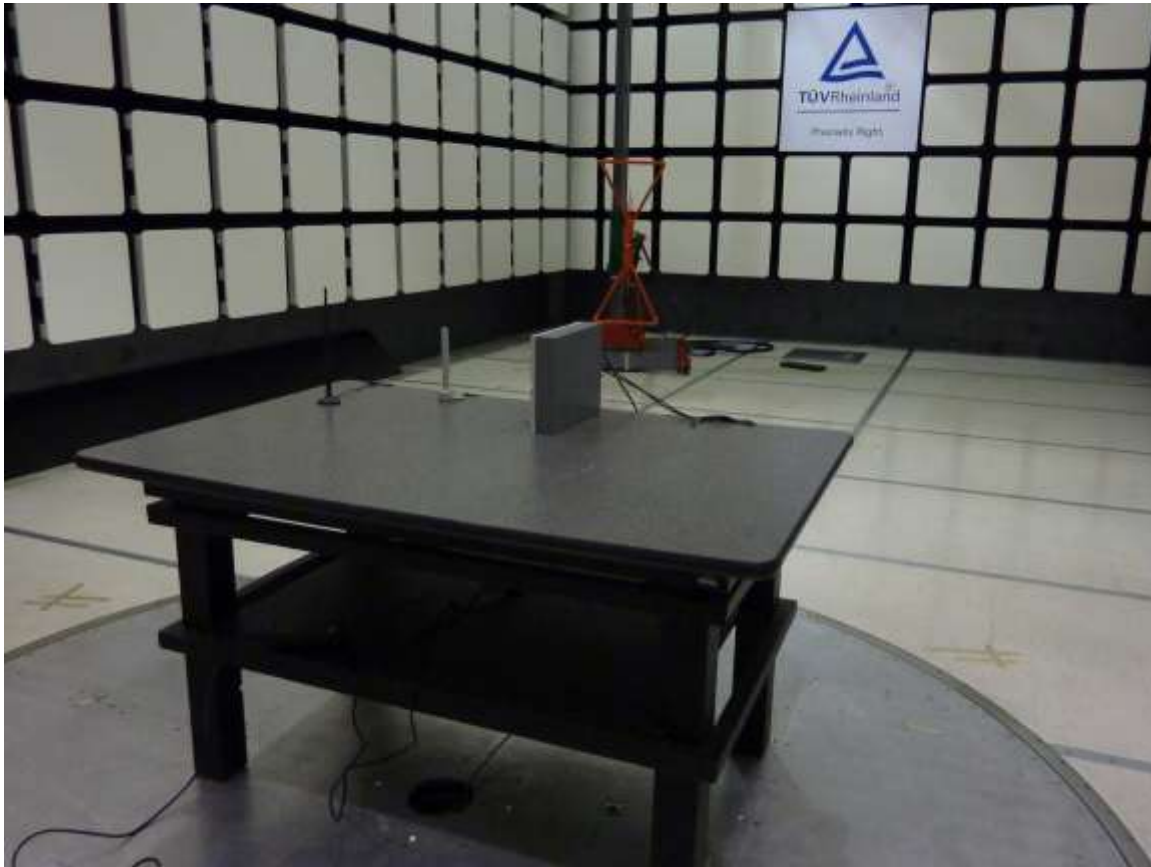
Test Setup – Radiated Emissions Normal and co-location operation
