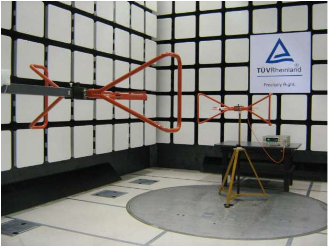
Photo of Test Setup for 30 MHz to 1000 MHz Substitution
