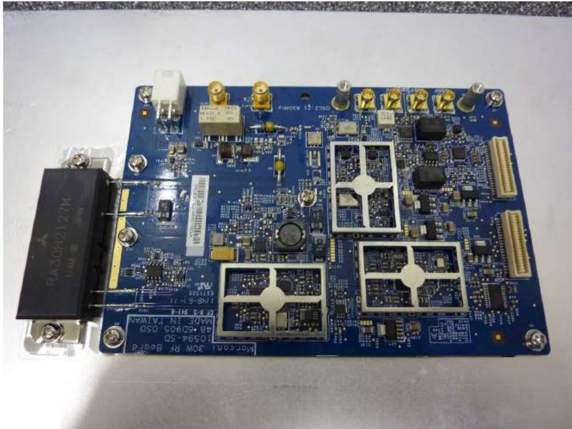
PTC Board Shields removed
