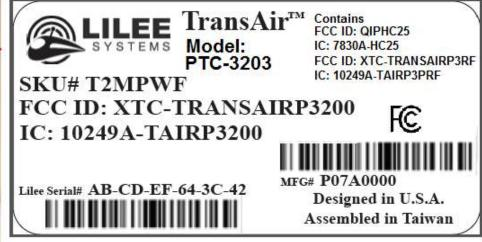
It will be put on with an adhesive on the back of the sticker. Some of the requirements for this sticker are that it can't be thorn/break in several pieces, resistant to fog, silver underside, waterproof, anti-oil pollution> 0.1 mm, and made from UL 94/VTM fire.
