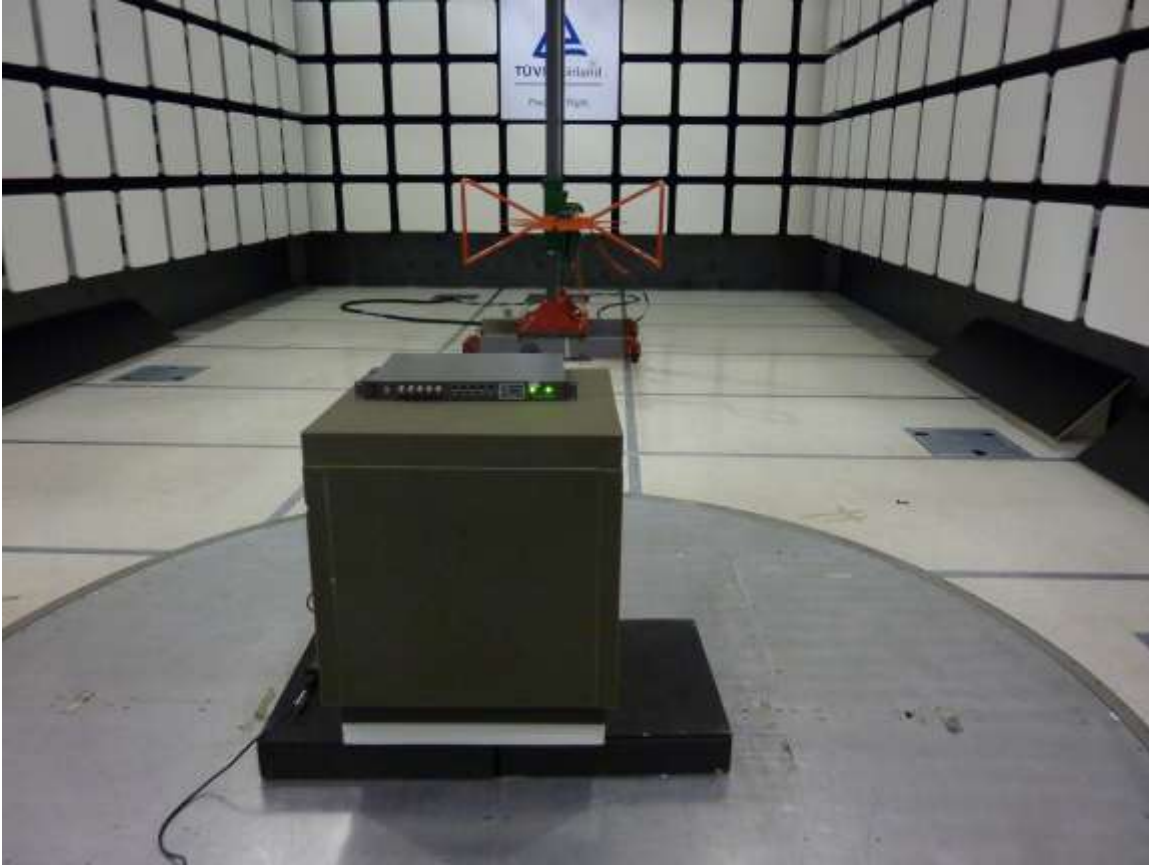
Test Setup – Radiated Emissions
