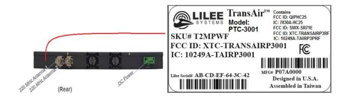
It will be put on with an adhesive on the back of the sticker. Some of the requirements for this sticker are that it can't be thorn/break in several pieces, resistant to fog, silver underside, waterproof, anti-oil pollution> 0.1 mm, and made from UL 94/VTM fire.
