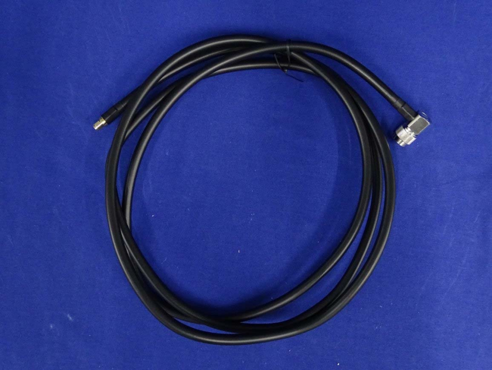
(28) EUT Photo (Patch Antenna Cable)
