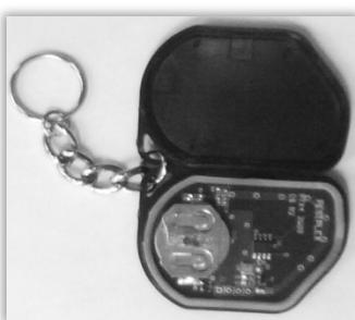
1. Carefully open the plastic case with a screwdriver from the key ring corner.
