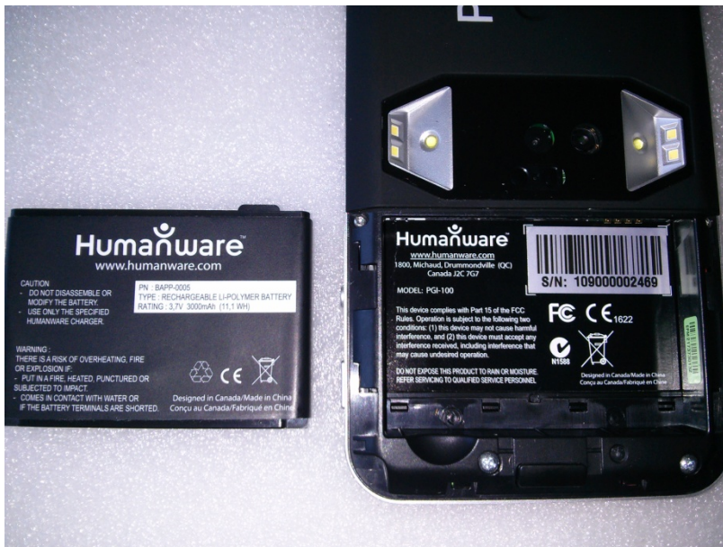
BATTERY REMOVED SHOWING LABELS LOCATION
