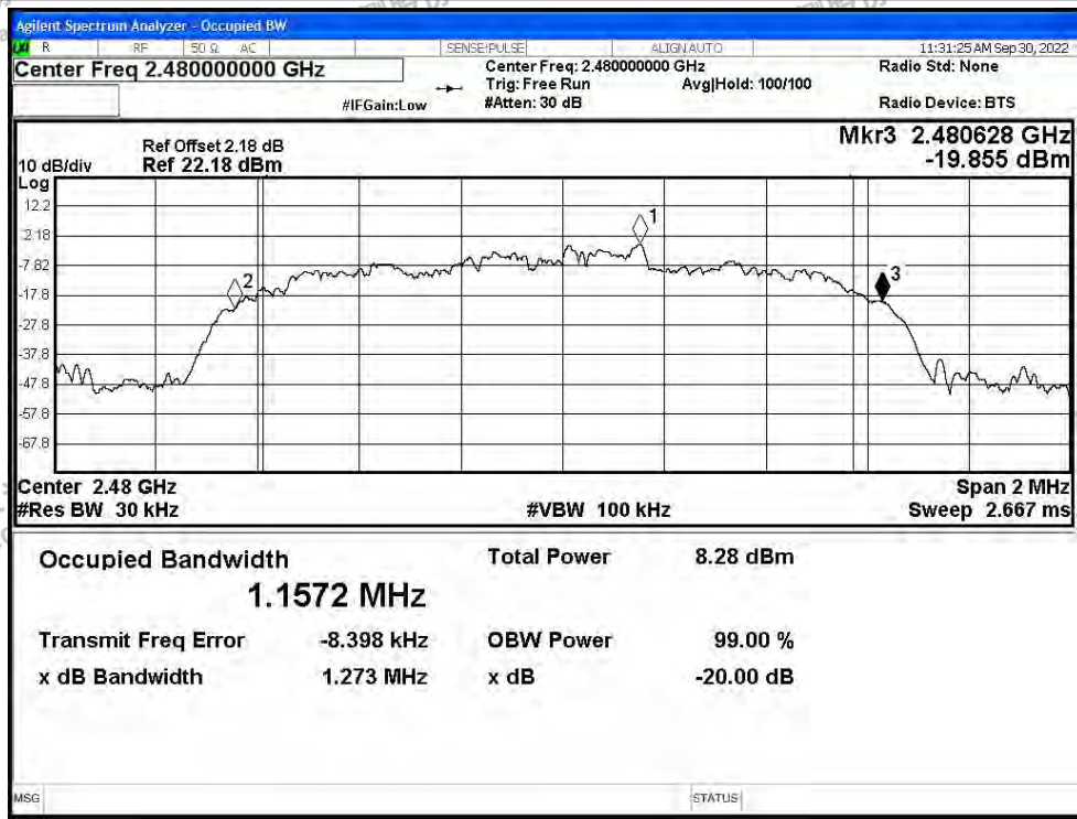
-20dB Bandwidth NVNT 2-DH5 2480MHz Ant1
