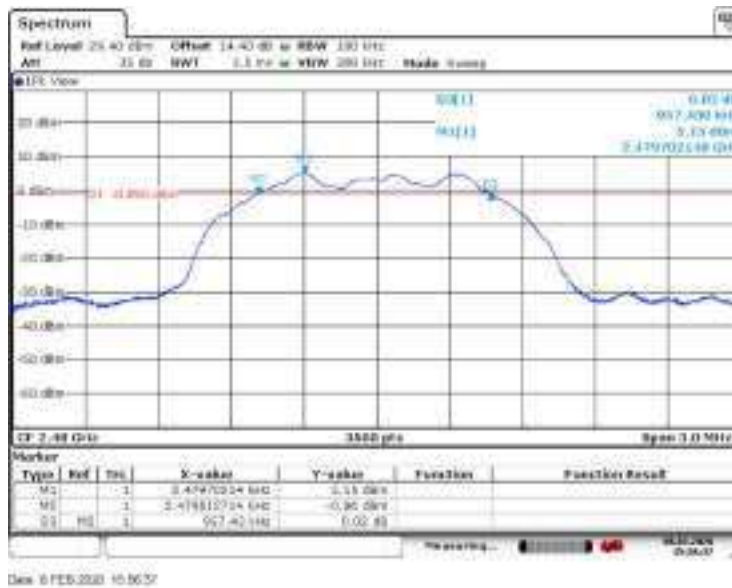
Figure 8.5-15: 6 dB bandwidth on high channel, sample plot
