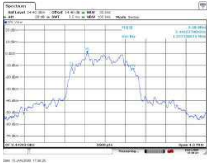
Figure 8.5-17: 99% occupied bandwidth on mid channel, plot
