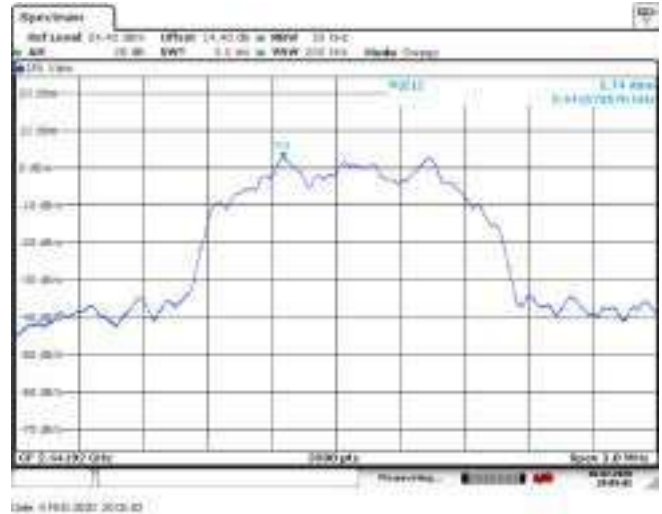
Figure 8.8-8: PSD sample plot on mid channel
