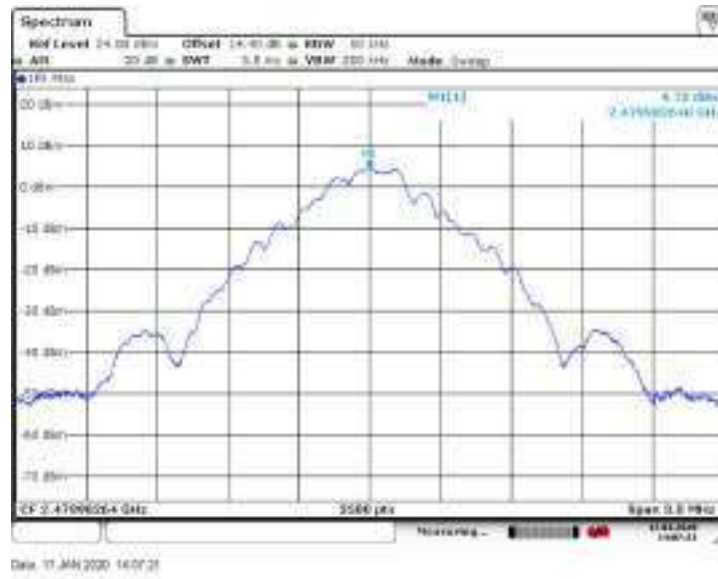
Figure 8.8-12: PSD sample plot on high channel
