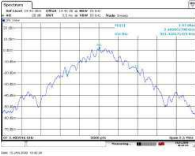
Figure 8.5-22: 99% occupied bandwidth on low channel, plot
