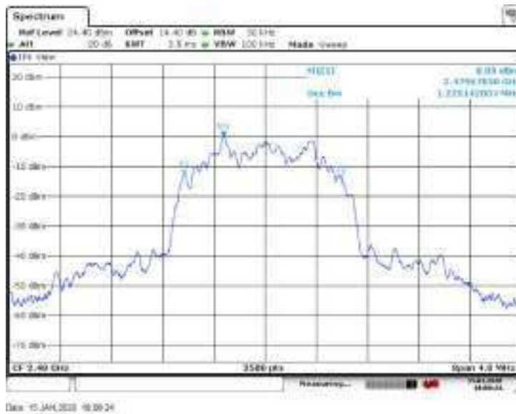
Figure 8.5-18: 99% occupied bandwidth on high channel, plot
