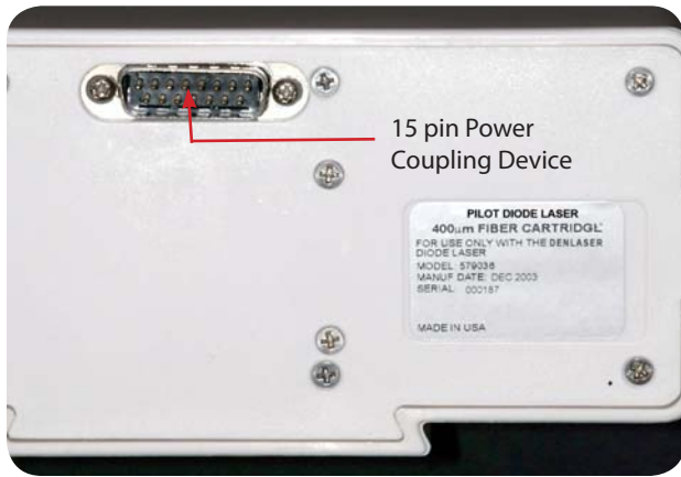
Figure 3.9 Base of the Fiber Cassette and the 15 Pin Power Coupling Device.
