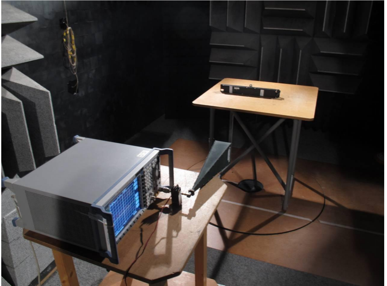
Photograph 5: - 3SM S01 WW, test setup radiated emissions (13-26 GHz)
