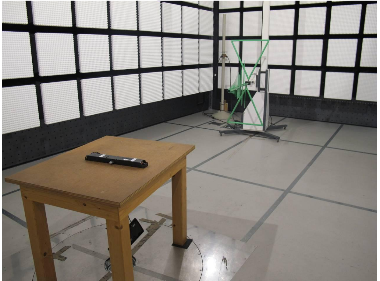
Photograph 2: - 3SM S01 WW, test setup radiated emissions (30 - 1000 MHz)
