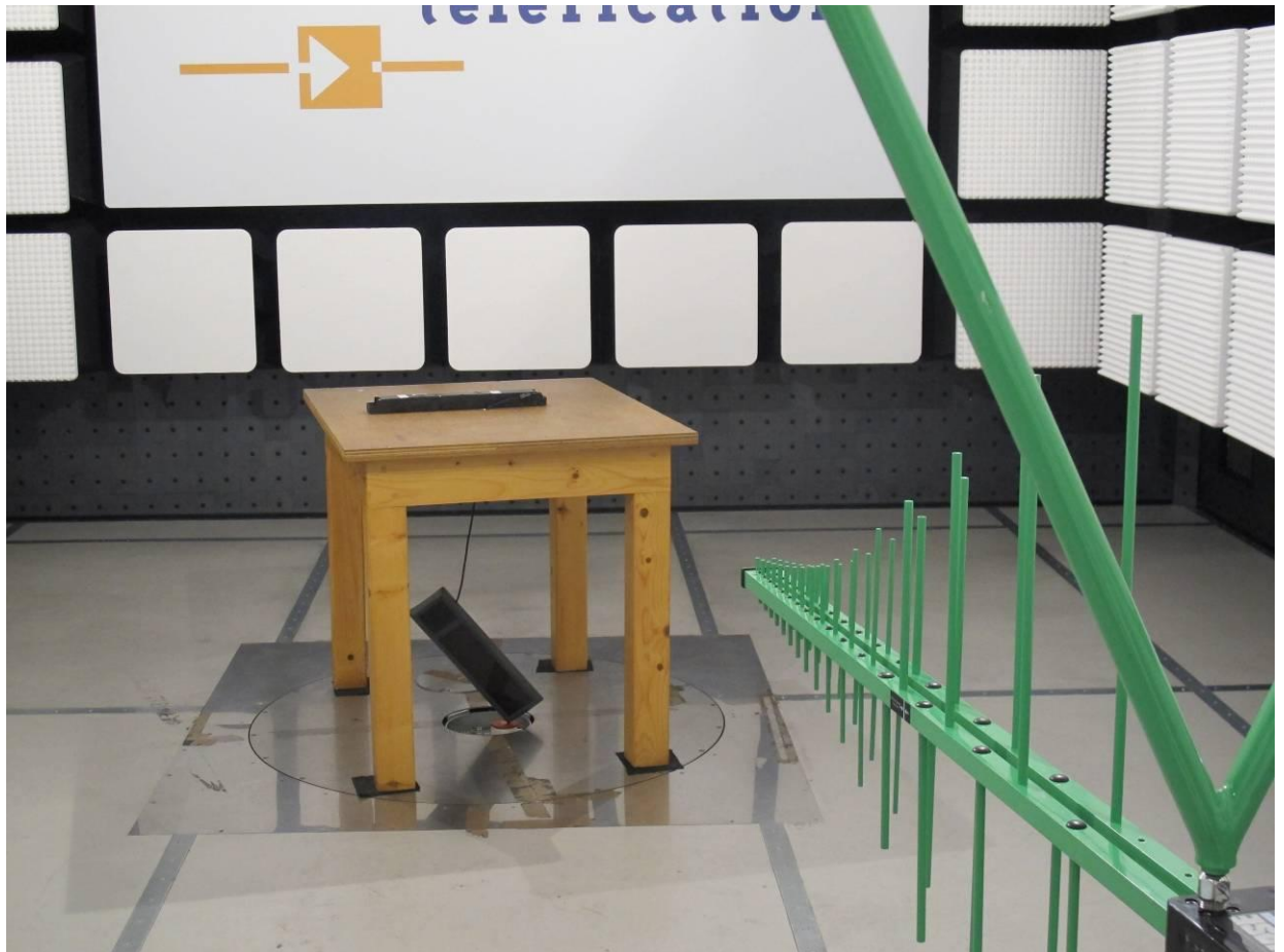
Photograph 1: - 3SM S01 WW, test setup radiated emissions (30 - 1000 MHz)
