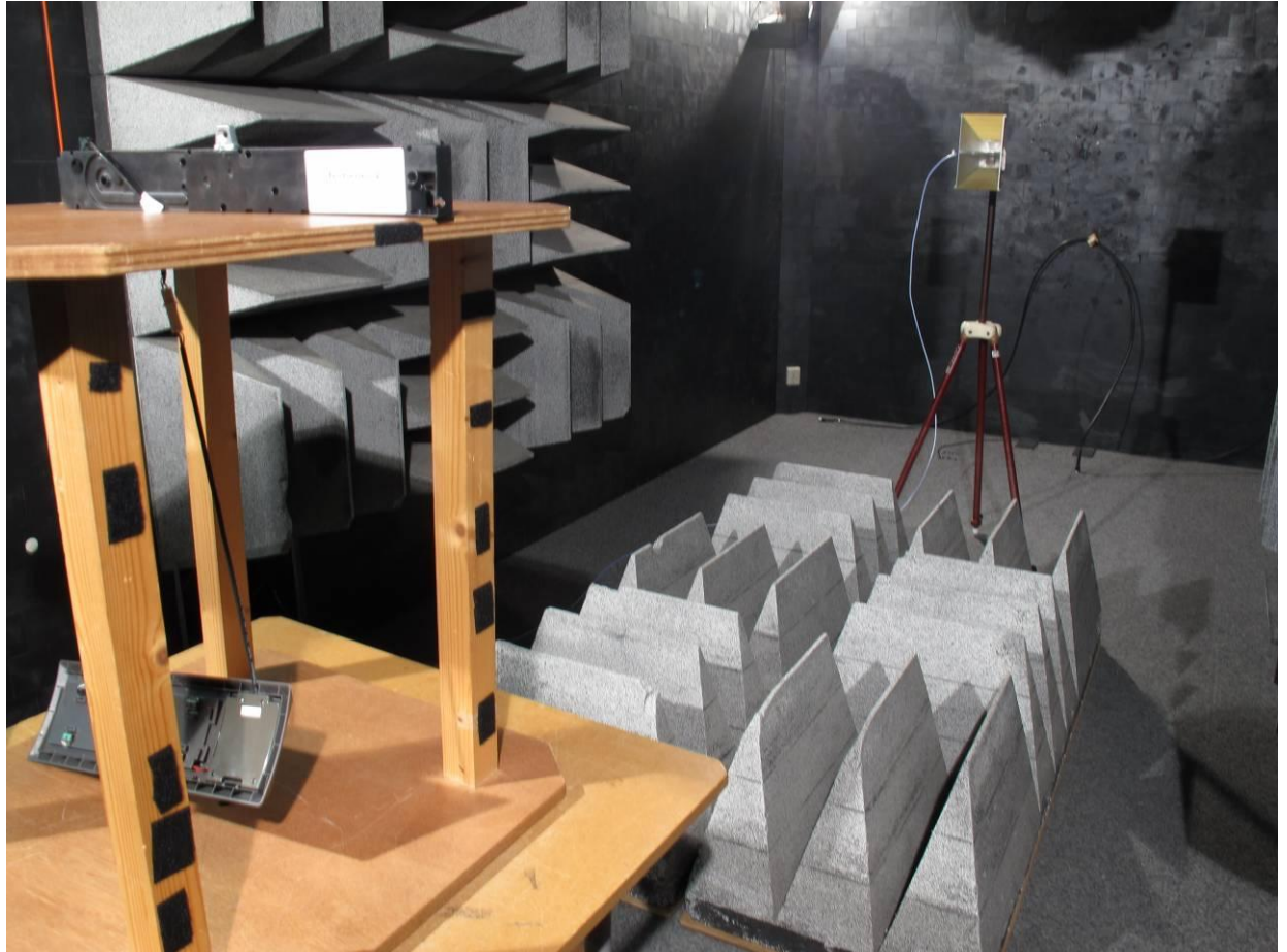
Photograph 4: - 3SM S01 WW, test setup radiated emissions (1 -13 GHz)
