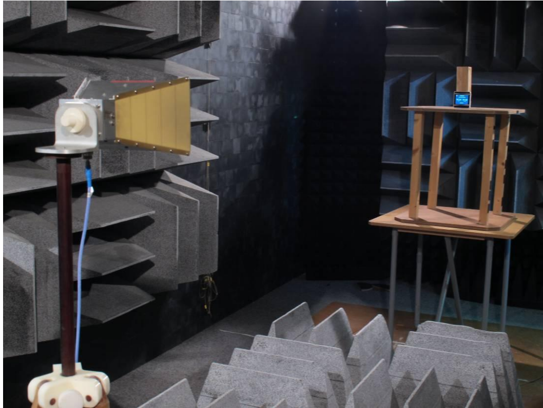
Photograph 3: - 3LR A02 US, test setup radiated emissions (1 - 18 GHz)
