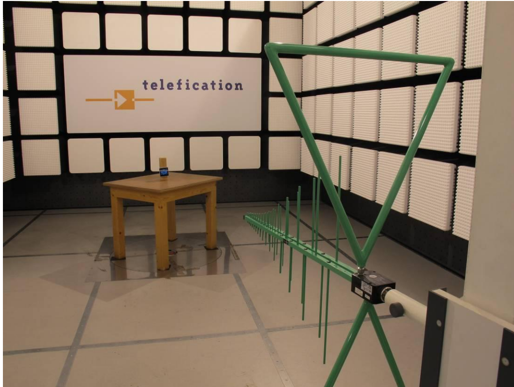
Photograph 2: - 3LR A02 US, test setup radiated emissions (30 - 1000 MHz)
