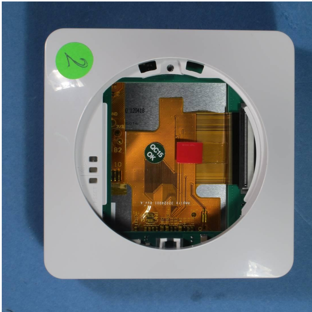
Photograph 2: - Velux 3LR A02 US, PCBinternal view 2
