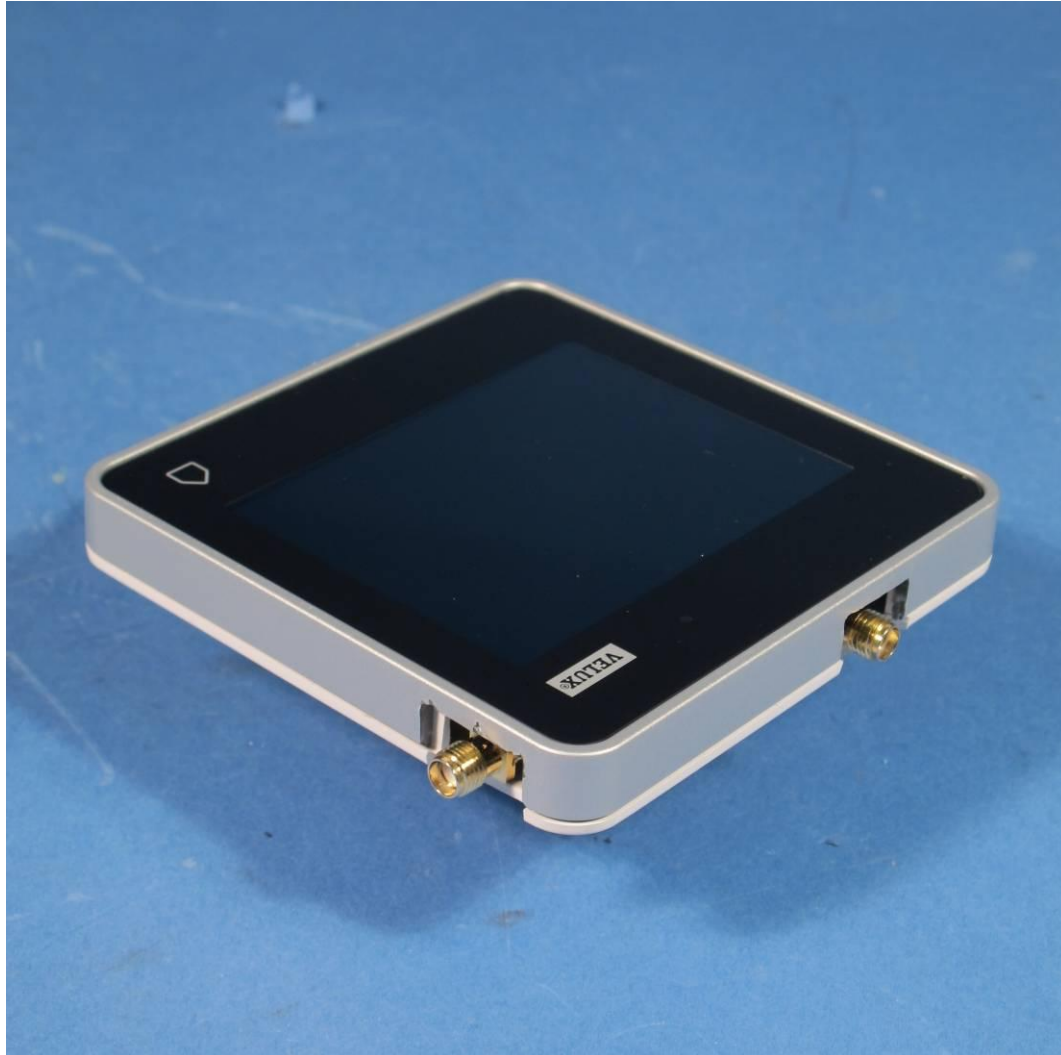
Sample for conducted RF measurements on antenna port.
