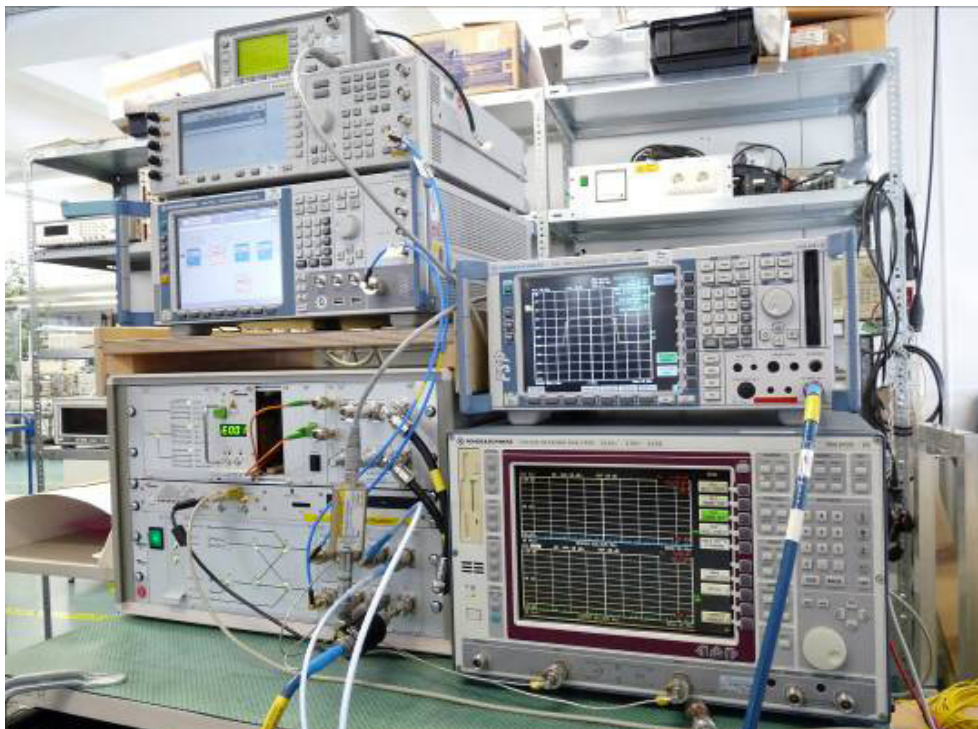
Test set-up for the conducted RF Tests
