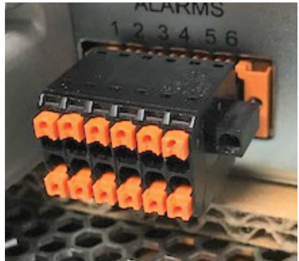
Mating connector inserted into WCS alarm port
