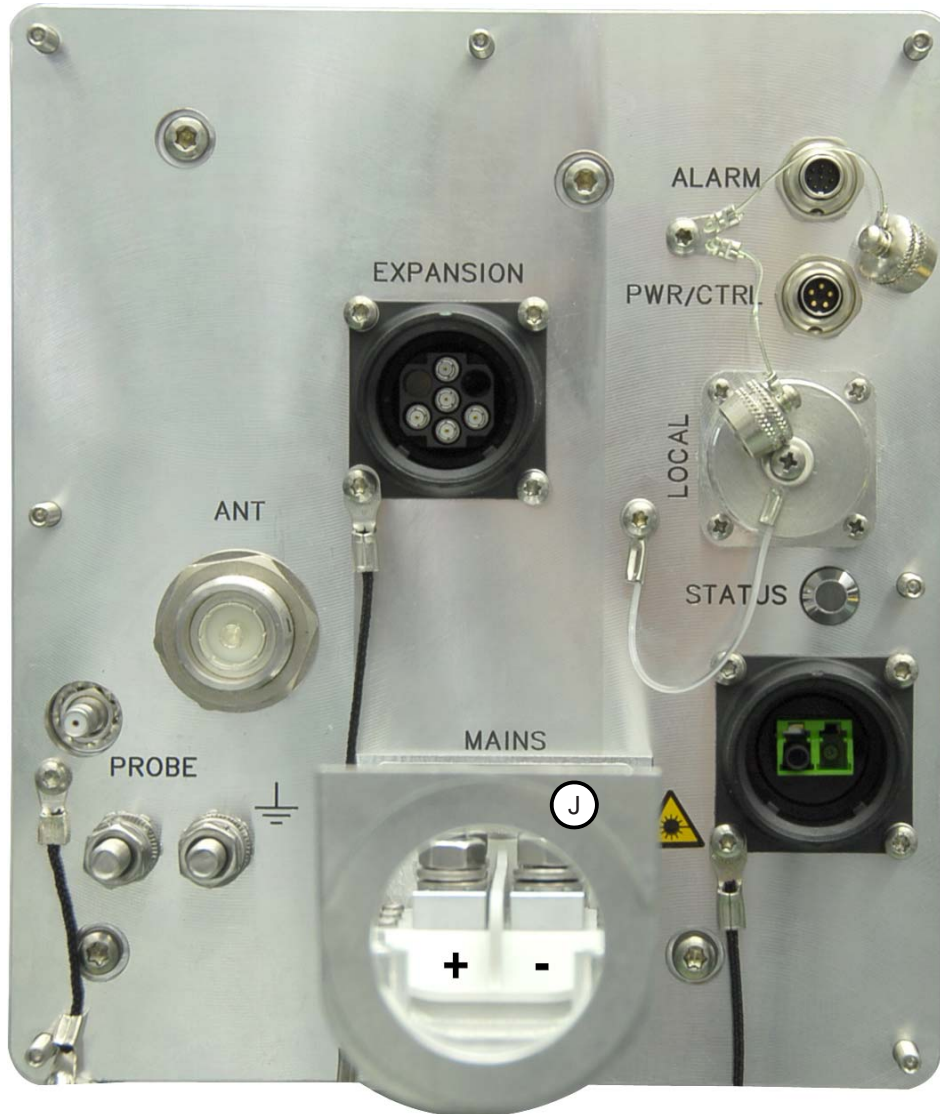
figure 4-11 ION-U H 7P/80-85P/17(E)P/19P DC version connector flange
