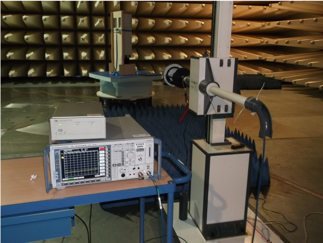
picture 8.4: Test setup: Field Strength Emission >1 GHz @3m in the SAC
