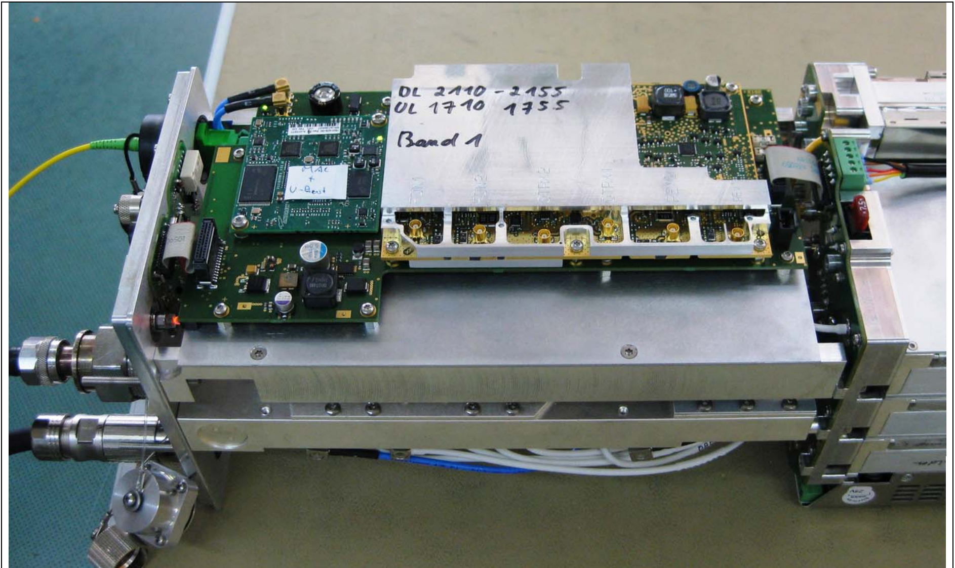
ECPD+, Control Board and Application Board
