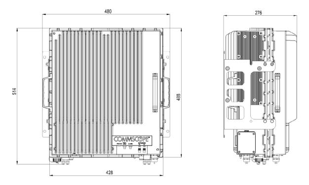
figure 6-4 Installation drawing of ION-U L Unit dual
