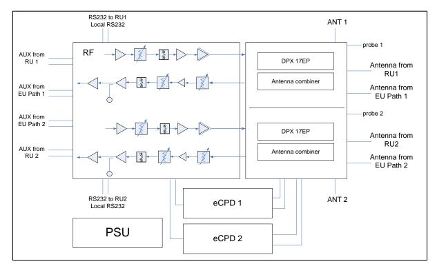
figure 3-1 ION-U EU L 17EP/17EP block diagram
