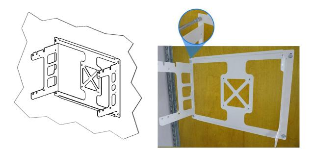
figure 4-1 Mounting bracket
