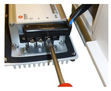
figure 5-5 EU power supply input cable
