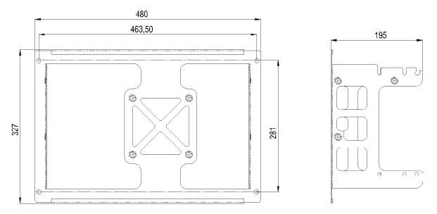
figure 6-1 ION-U Low Power EU mounting bracket
