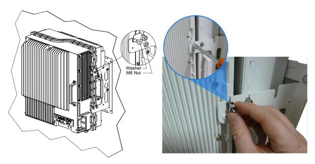
figure 4-15 Attach M6 nut to threaded pins for 2<sup>nd</sup> unit
