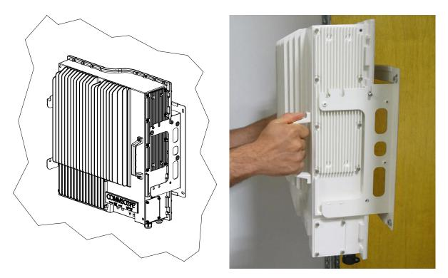
figure 4-6 Place EU onto wall mounting bracket – single mount
