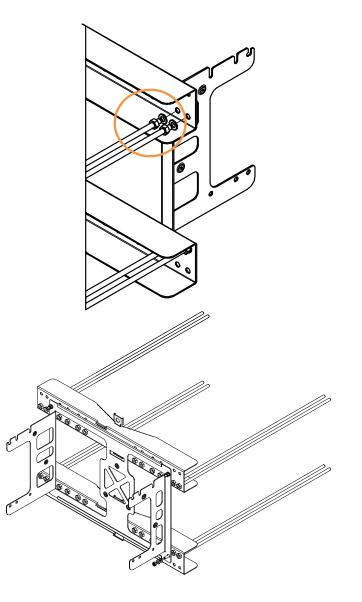
Mount the pole-mounting kit with the two brackets and M8 plain washers (5), split lock washers (6), and self lock nuts (7) to the pole.
