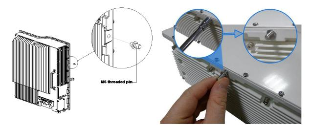
figure 4-4 EU threaded pin power supply side
