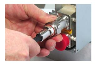
5. Retain the cable connector with the counter wrench and fasten the coupling nut with the Torque wrench torque wrench until the torque is applied (torque wrench clicks).
