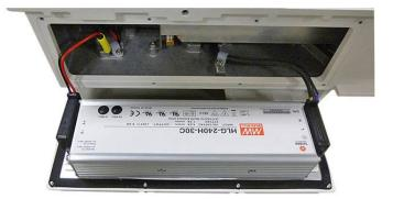
figure 5-4 EU power supply with cables
