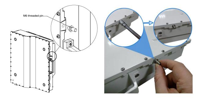
figure 4-5 EU threaded pin narrow side
