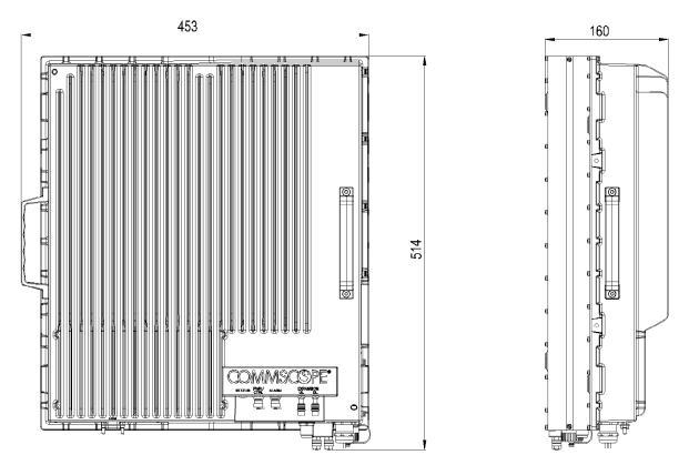
figure 6-2 ION-U Low Power Unit dimensions
