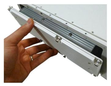
figure 5-8 EU with replacement power supply
