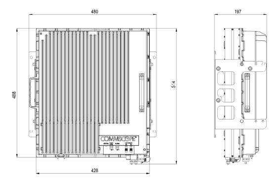
figure 6-3 Installation drawing of ION-U L Unit single
