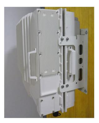
figure 4-16 Completed dual unit mount
