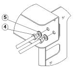
3. Screw the end of the threaded bolts (with the nut and washer) from the inner side to the welded nuts of the polemounting bracket. Use the nuts that allow to mount the mounting kit with the threaded bolts as close to the pole as possible. Lock the screwing by fastening the M8 nut.
