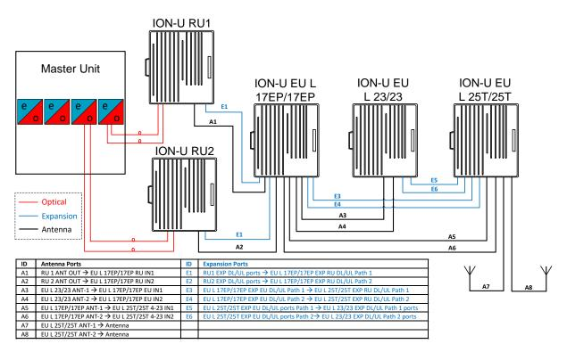
figure 3-8 Two RUs three EUs (RU band loss minimized) RF
