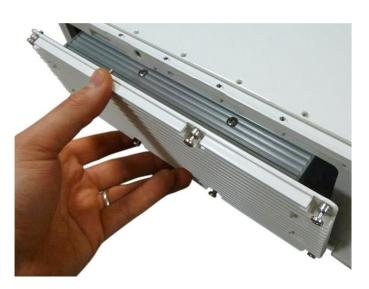
figure 5-9 EU insert power supply
