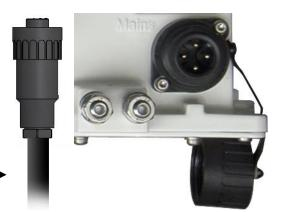
figure 5-1 Disconnect mains power
