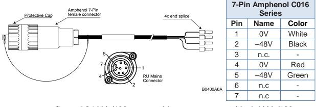
figure 4-21 Vdc/100 power cable
