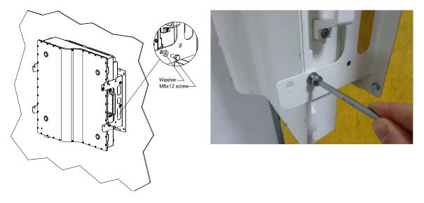
figure 4-11 Install M6x12 screws and washers
