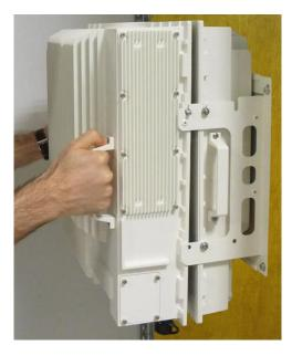
figure 4-13 2<sup>nd</sup> unit on wall mounting bracket
