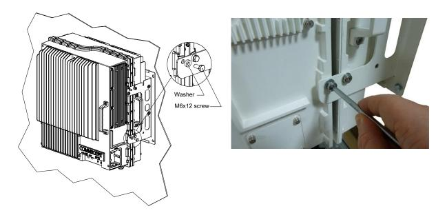
figure 4-14 Install M6x12 screws and washers 2<sup>nd</sup> unit
