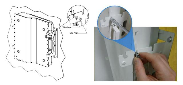
figure 4-12 Attach M6 nut to threaded pins
