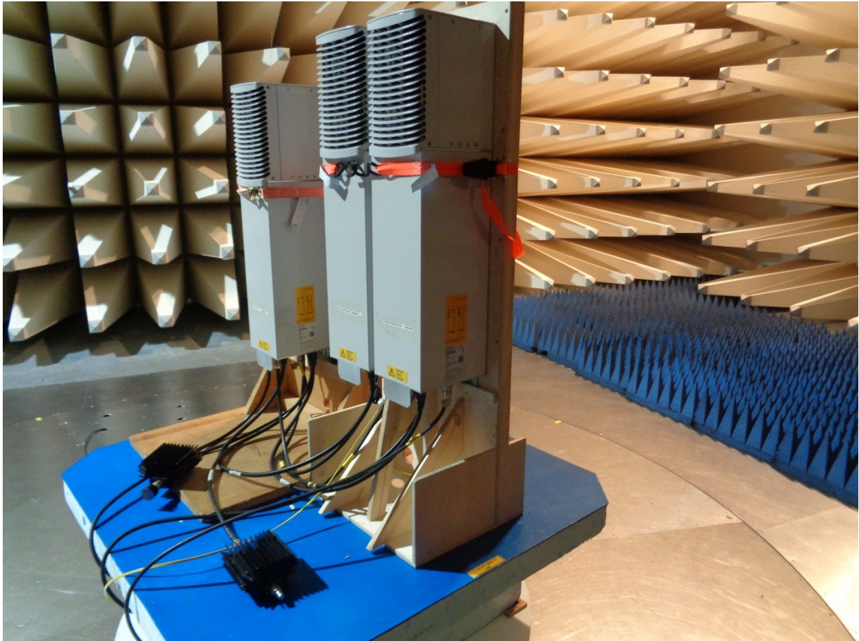
picture 8.5: Test setup for one band (test configuration 1)
