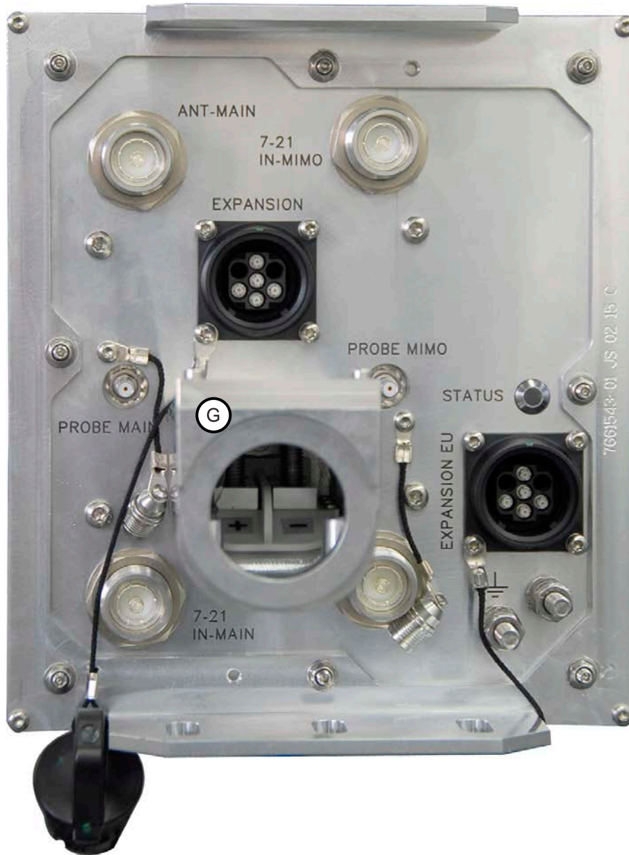
figure 4-12 ION-U EU H 23/23 DC version connector flange
