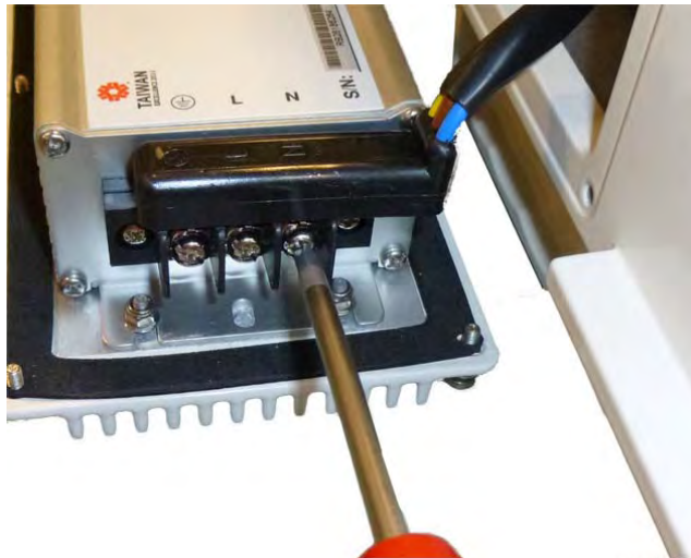
Figure 4-95 RU power supply input cable
