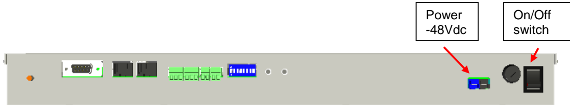
Figure 6-14 Rear view of the TPRF31 Fast MiniRack: Power supply connectors and On/Off switches
