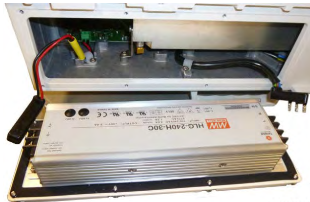
Figure 4-96 RU power supply output cable
