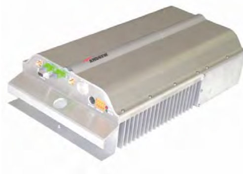
Figure 4-4 Case R2E Remote Unit
