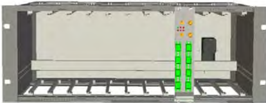
Figure 6-33 Installing a TFLN module
