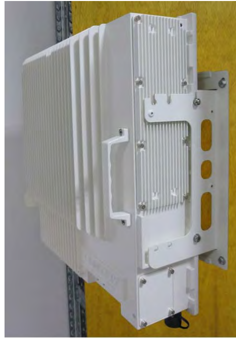
Figure 4-76 Completed RU Mount
