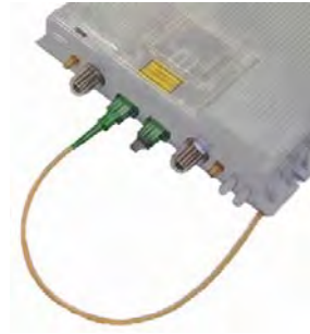
Figure 4-8 Correct handling of optical connections with ION-B RUs
