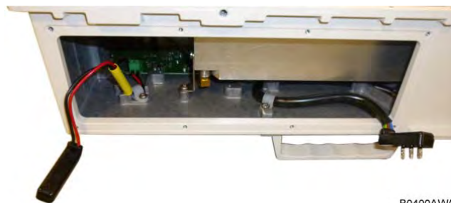
Figure 4-97 RU with power supply removed
