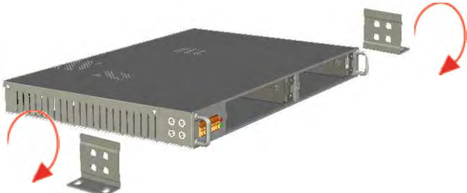
Figure 6-24 Turning the brackets
