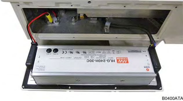
Figure 4-94 RU power supply with cables
