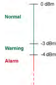
Figure 6-36 AGC thresholds vs LED alerts
