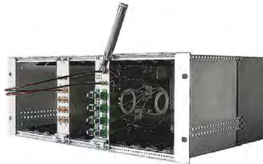
Figure 6-34 Proper cabling of SMA connectors on a TFLN front panel
