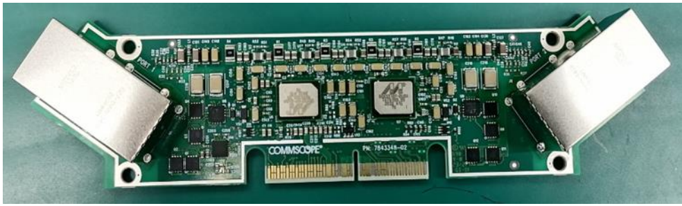
DPEM 1 - 7843349-02 – Data & Power Entry Copper – TOP View
