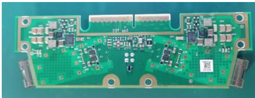
DPEM 2 - 7843351-02 – Data & Power Entry Fiber – BOTTOM View
