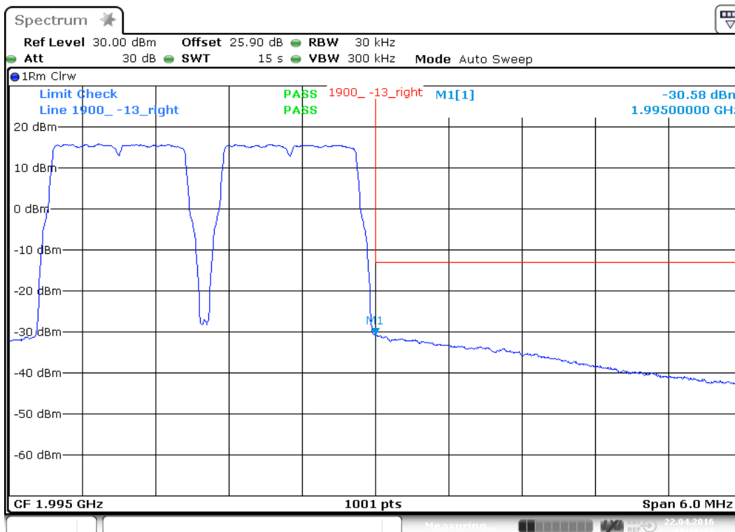
plot 8.3.1.5-#1 Intermodulation: §24.238, §2.1051; Test results; Downlink; LTE Lower Band Edge
