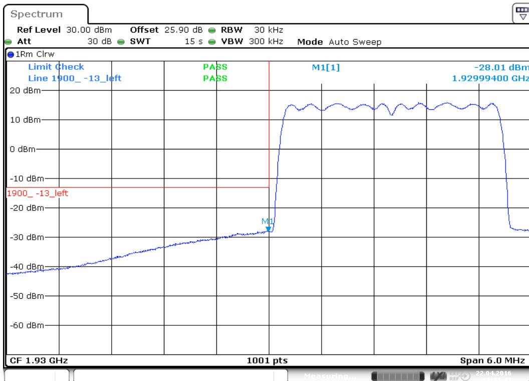
plot 8.3.1.3-#1 Intermodulation: §24.238, §2.1051; Test results; Downlink; CDMA Lower Band Edge
