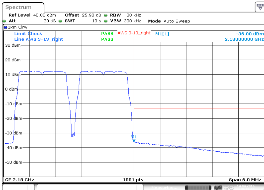
plot 8.3.1.3-#1 Intermodulation: §27.53, §2.1051; Test results; Downlink; LTE Lower Band Edge
