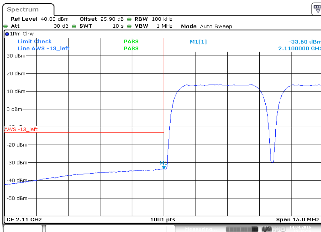
plot 8.3.1.2-#1 Intermodulation: §27.53, §2.1051; Test results; Downlink; WCDMA Lower Band Edge
